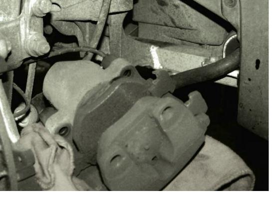
Always support the caliper after removal. This allows you to easily change the pads and takes the tension off of the flexible brake line and/or the brake lining sensor wire.
