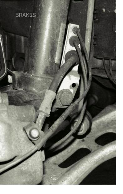
Make sure the brake lining sensor wiring is properly secured. This will prevent the wire from rubbing against anything and possibly turning the light back on.
