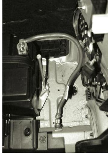
Notice how the battery ground cable is bolted directly to the frame. This is important since another ground cable is mounted between the engine and the frame at the front of the vehicle. This forms the ground path for the starter. Remember, when doing voltage drop testing always connect your ground test lead directly to the negative battery post only!
