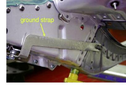
On certain vehicles where the front end is aluminum and the rest of the body is steel, ground straps like these are necessary to ground the two parts. There is no weld to form the ground path, and the structures are bonded with adhesives and rivets (courtesy Collision Industry Conference).
