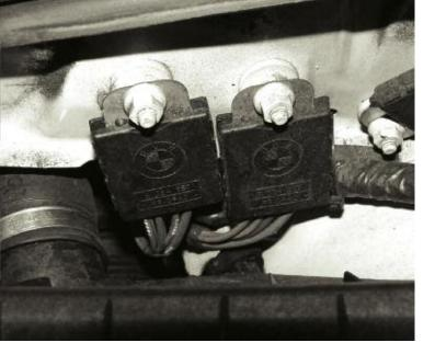
Here we have multiple ground connections attached to an inner fender support. As the fender is asked to ground numerous electrical components, you need to insure the fender is properly grounded to the rest of the body in order to handle the load.
