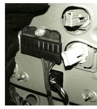
This ground for the rear lighting is mounted to the trunk support frame. These are often steel panels that are spot welded to the rest of the body. Since the metals are the same, the weld forms the ground path.
