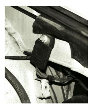
This is not an electrical device, but a multiple ground point. All those brown wires are connected together on a buss bar inside the black plastic cover. This is bolted to the inner fender and forms the ground path for multiple items.
