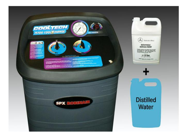
Here is a tool that might be a good investment providing you sell enough cooling system services. You can keep one tank with a 50/50 mixture of Mercedes-Benz coolant and distilled water and exchange it with the old coolant without even running the engine. You may still have to pump out the heater cores separately.
