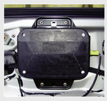
This is a driver's door airbag on an ML series. Notice how the unit is riveted in to provide clearance for the window, so nuts and bolts should not be used as a substitute.
