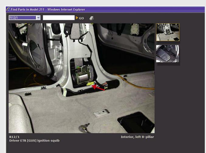
With a paid subscription to www.startekinfo.com, you can access information such as component location of the driver's seat ETD found mounted here in the B pillar. These units have a pyrotechnic charge that fires and applies tension to the belt even if the airbags do not deploy.
