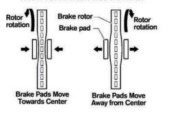
Disc Thickness Variation causes pedal pulsation as the "fat" spots pass between the pads.
