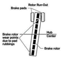
Runout makes the rotor wear unevenly as high spots hit the friction material.
