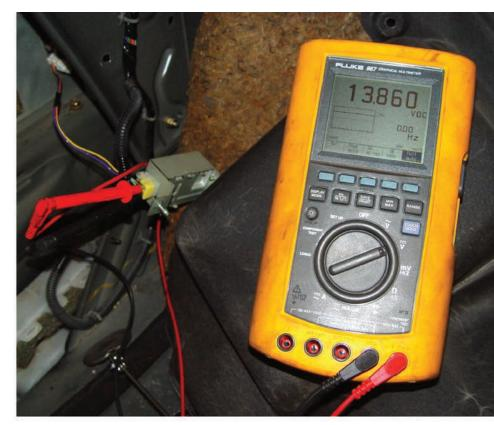
You can measure voltage at the pump control module, which is mounted in the trunk. In this case, the relay is providing 13.8 volts and the module is grounding the pump completely to get maximum output.
