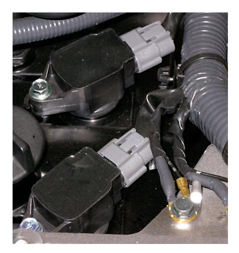
(TDC). Distributors, rotors, and spark plug wires have mostly been replaced by Coil-On-Plug (COP) technology, which Nissan was one of the first to employ.
