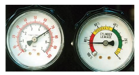
A cylinder leakdown test can tell you more than you've found out from a compression test. Listen for escaping air, look for bubbles.
