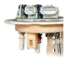
If fuel pressure is not up to spec, it doesn't necessarily mean the pump is bad. In this assembly, you can see green copper oxide corrosion forming in the wiring to the pump, which causes high resistance and poor pump performance.
