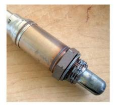
If any appreciable amount of coolant has been passing through a cylinder or two because of a leaky head gasket, there is a good chance that the O2 sensor(s) has become contaminated and will only send a "lazy" signal.
