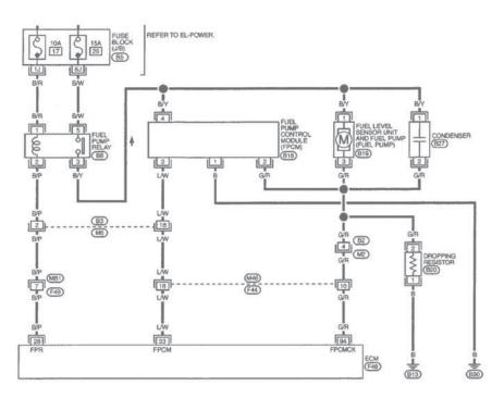
Here is a wiring diagram of a fuel pump control module on a 2000 Nissan Maxima. The module receives a signal from the PCM. Depending on this signal, the module either grounds the fuel pump directly, or allows it to ground through the dropping resistor only.
