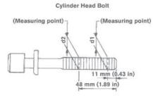
Never reuse "plastic zone" or "torque-to -yield" head bolts without comparing the diameters of the threads at the points shown. If the difference is larger than the specification, get new bolts or risk twisting one off and ruining your schedule.
