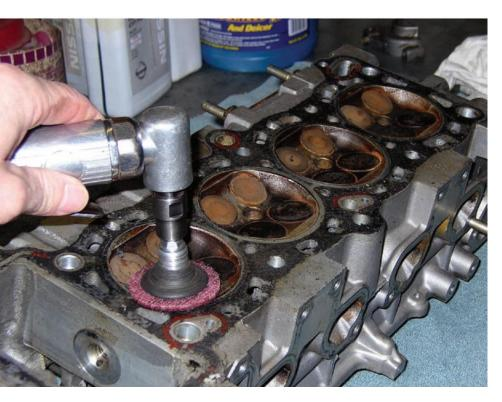
Applying an aggressive "zip" disk to the head is NOT recommended. Not only can it make dents and waves much faster than you might expect, it will contaminate the engine with abrasives that may damage bearing surfaces.
