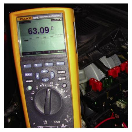
To see if the CAN lines have an electrical problem with the wiring you can get access to the CAN lines (there under the fuse box in a 140 chassis) and measure resistance between CAN low and CAN high. Since there are two terminating resistors in the circuit in two of the control units you should measure about 60 ohms.
