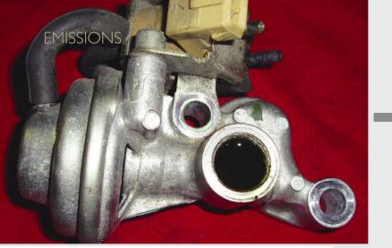
The EGR valve and solenoid are sold as one unit. The large threaded opening is where the pipe that leads to the intake manifold attaches. The liquid inside is carbon cleaning solution.
