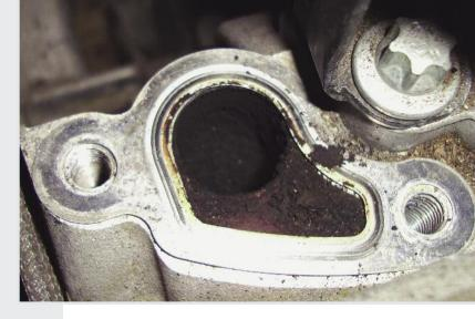
Block this EGR passage to eliminate the possibility of any exhaust making it into the intake manifold. If the engine runs smoother, you have a leaking EGR valve. Verify that it is not being opened by vacuum from a solenoid that's stuck.
