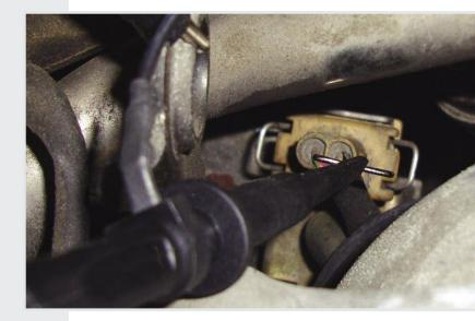
Here we are monitoring the ground control of the solenoid. A reading of I 2V means it is not energized and no vacuum will flow to the EGR valve. When the ME grounds the solenoid, the EGR valve should open.
