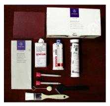
A kit is available through your Mercedes-Benz parts supplier that will allow you to bond panels using adhesives. Notice the two static mixers with pink tips. Before attaching the mixing tube, squeeze out one inch of material. After attaching the tube, squeeze out another inch to equalize the amounts.
