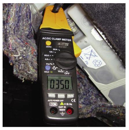
When testing for battery drain, look at amperage draw after the vehicle has been shut off for several minutes to be sure all the control units have gone to sleep. The normal procedure of unplugging fuses to locate the draw must be augmented by unplugging control units from the CAN for the same purpose.
