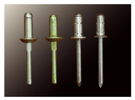
Mercedes-Benz requires all chemical bonding to be supported by some mechanical attachment such as spot welding. Or, when attaching dissimilar metals, you can use these special structural rivets, which are available from your Mercedes-Benz parts supplier.
