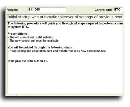
At this point, you need to have the old control unit still plugged in. Selecting "Initial startup of a new control unit" will lead you to this screen. Follow the directions and the existing coding will be read from the old unit.
