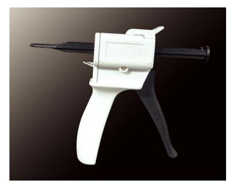
see an adhesive compound mixed with a hardener similar to that used with body filler. This chemical reaction usually occurs best at 75 deg. F. and will take about an hour or somewhat more to dry. It will take roughly four hours to fully cure, but you can continue repairs after the first hour. Acrylics may dry faster, but their strength limitations should limit them to smaller repairs.
