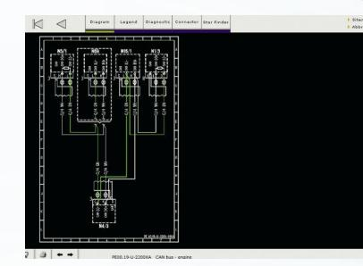
This is a wiring diagram of one of the first Mercedes-Benz CAN systems, including control units for the powertrain. The DI/KSS (N1/3 ignition), LH-SFI (N3/1 fuel injection), CC/ISC (N4/3 Cruise & Idle), TCM (N15/1 transmission) and Diagnostic Module (N59 OBD I) are all communicating on this network.
