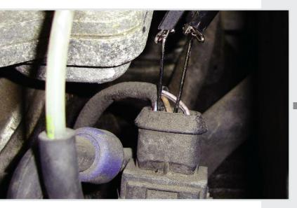
The MAP sensor is only used to diagnose emissions-related systems such as EGR and EVAP flow issues. You can use the MAP to monitor manifold vacuum and the open the EGR valve. Watching the change in the vacuum reading will tell about the flow of the EGR system.
