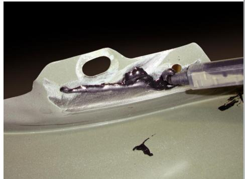
You are not limited to using chemical bonding only on panels that are not bolted or riveted.
