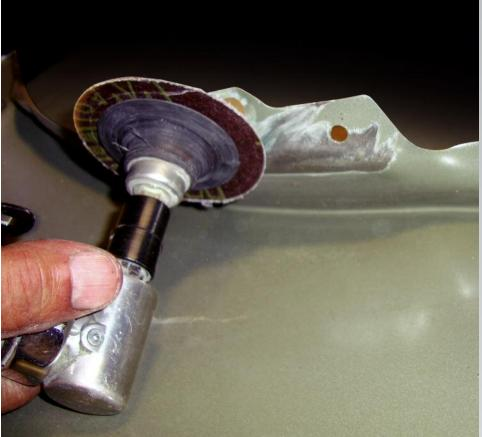
Follow the adhesive manufacturer's instructions for surface preparation. Metal panels may need to have their galvanic coating removed before the panel is applied to the structure. At the same time, care needs to be taken not to compromise corrosion resistance at the repair area.
