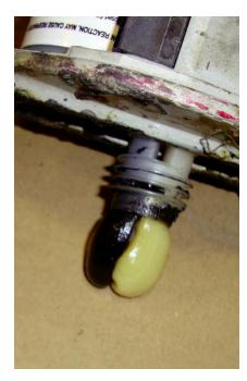
First, squeeze one inch of bonding material out of the tube, then install the static mixer and discharge another inch to "equalize" the mixture. This will ensure equal and properly mixed adhesive material.
