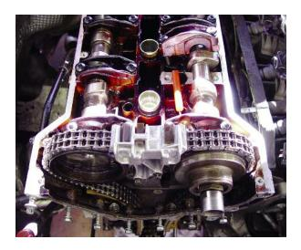
On this 111 engine, if the camshafts are in their home position you will be able to install a cam positioning tool in the backs of the cam sprockets. The screwdriver indicates the location of one of the holes (intake cam). Notice how the intake and exhaust cam lobes are facing one another. This gives you a ballpark idea that you have the timing close.
