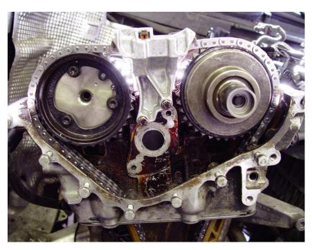
Look at the intake cam on the right and you can see the camshaft timing adjuster. Since the engine rotates clockwise, you need to turn the adjuster counter-clockwise all the way until it stops, then engage the timing chain.
