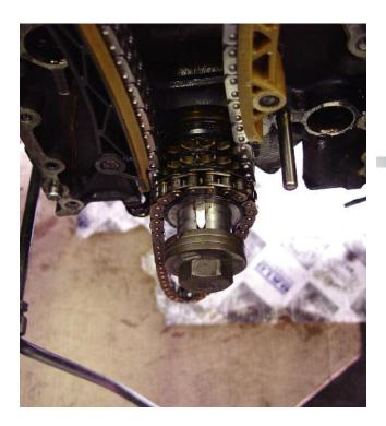
Mercedes-Benz usually times its engines at a position other than TDC. In the case of this 111 engine, the timing pulley should be set to 20 deg. after TDC. This puts the keyway in the crankshaft at just about the 12 o'clock position. Now, you should be able to line up the cams.
