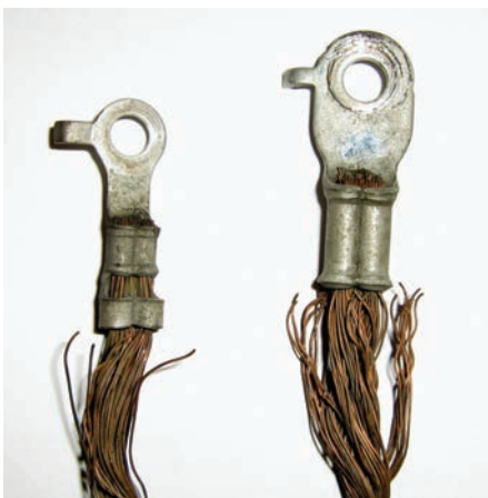
| Figure 4 Frayed ground straps can cause voltage drops on the negative side of a circuit.
