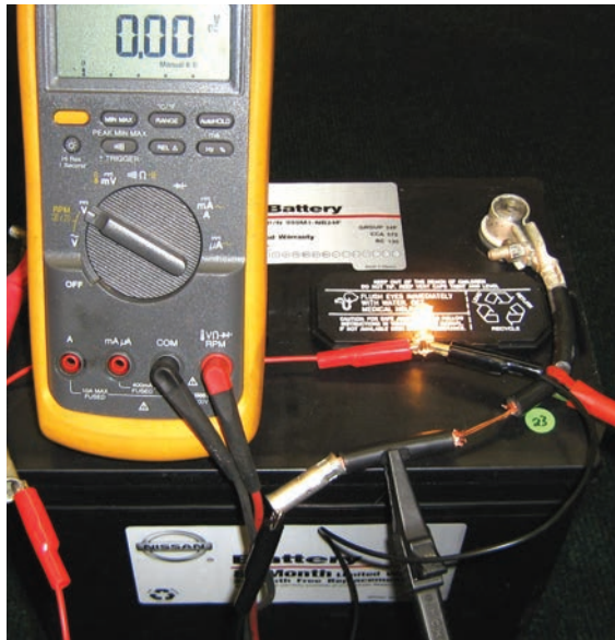
| Figure 2 The cable carries enough current to light up a small bulb.
