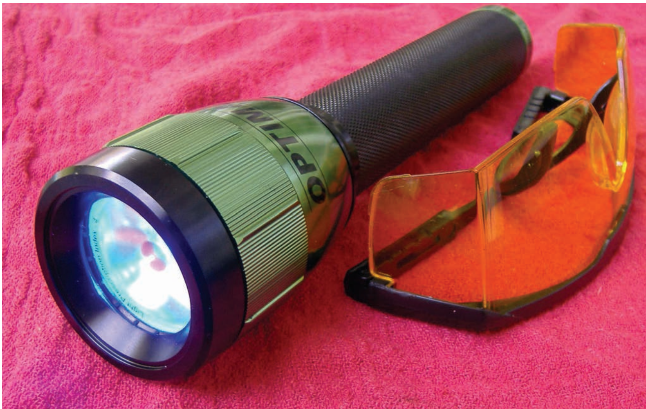
| Figure 1 – The Nissan/Infiniti-recommended UV method is a great way to find leaks, but make sure you use a dye formulated to work with water-based fluids, such as Part Number J-29545-6A.
