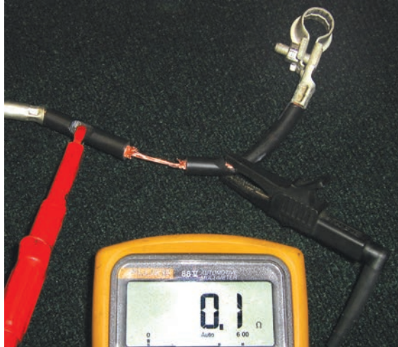
| Figure 1 This battery cable has been altered to simulate internal damage
