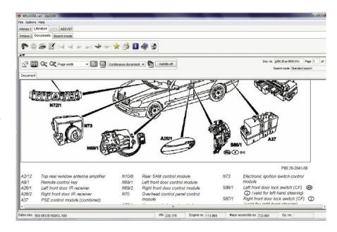
one quick tip, however: If the vehicle has an EDW alarm system, you can disconnect the intermediate plug of the EDW cable harness from the connector (M14/1x2, or M14/2x2) and connect the central locking cable harness directly to the supply pump. If central locking works okay now, it's time to delve into the EDW.
