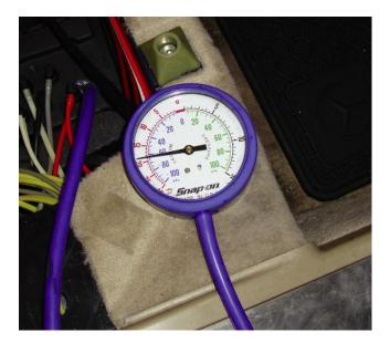
The PSE module contains its own vacuum/pressure pump. Vacuum is used to lock the door. You can monitor the vacuum supply with a gauge while commanding the system to lock. A good pump and pull almost 20 in. Hg.
