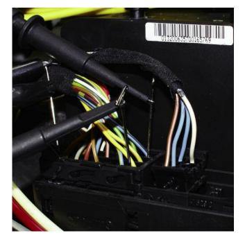
By monitoring the SN1 and SN2 signals, you can evaluate the command to the PSE module to both lock and unlock the doors. You do not need to use an oscilloscope to monitor these signals. A DMM will work fine. You are looking for a 12V signal on each of these wires.
