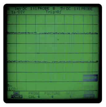
Looking at these signals on a dual trace scope allows you to see the lock command (upper trace) and unlock command (lower trace). As you can see, the 12V signal gets pulled to ground when the door locks are actuated, in this case by the RCL unit as the remote button is pushed to open and close the doors. The signals are there, but the pneumatic pump did not turn on. At this point, check for powers and grounds to the PSE unit. If they are good, replace the PSE module.
