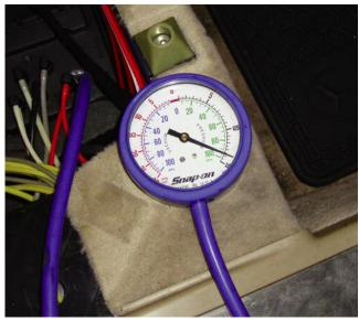
The same line that supplies vacuum to the individual door lock actuators also supplies pressure. A good pump can produce almost 1.0 bar (14 psi). Of course, an air leak will decrease both vacuum and pressure.
