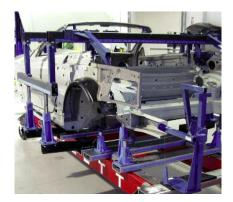
Here is a Celette bench with a 230 chassis set up for measurements and pulling. The framework setup and procedures are all available on the website. Remember, you can use higher strength steels to pull lower strength steel, but you cannot reverse the rule.
