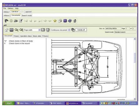
With a paid subscription to www.startekinfo.com, you can use WIS-Net to pull up the K-point measurement data. This information is only used for diagnostic purposes, particularly on older models built before the turn of the millennium. You can use these measurement points to see how bad the damage is.
