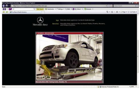
Car Bench is a Mercedes-Benz approved alignment jig for frame straightening. There are various models available, and by visiting www.carbenchna.com you can arrange bench rental and download measurement specifications.
