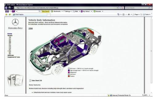
Before you start the pulling process you need to know what metals you are working with. Mercedes-Benz uses different metals with different strength levels to achieve structural strength and occupant safety. A visit to www.mbcollisioncenters.com and your membership gets you this important data.
