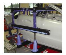
Here is a frame attached to the bench. Points on the chassis can be measured from here, and you can start the pulling process. On this 230 chassis, you need to be aware of the different metals and their relative strengths.
