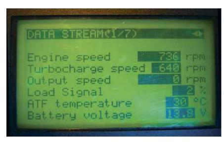
USE SCAN DATA TO DETERMINE TRANSMISSION TEMPERATURE. IF YOU DO NOT HAVE BMW SOFTWARE, YOU CAN ESTIMATE TEMPERATURE FROM ENGINE DATA. USUALLY AN ENGINE AT IDLE OVER SO DEG. C WILL HEAT UP THE TRANSMISSION FLUID TO ABOUT 30 DEG. C. ATF through the fill port until it starts to drip out.
