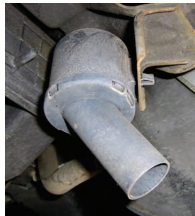
Figure 6 The water separator is the canister's fresh air intake.
