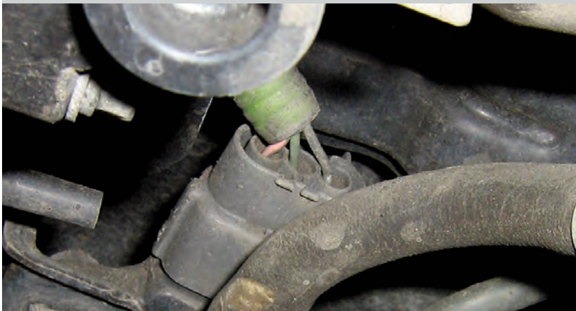
Figure 3 The fuel tank pressure sensor works like a MAP sensor.
