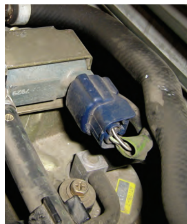
Figure 2 The purge valve is a duty-cycle controlled by the PCM
