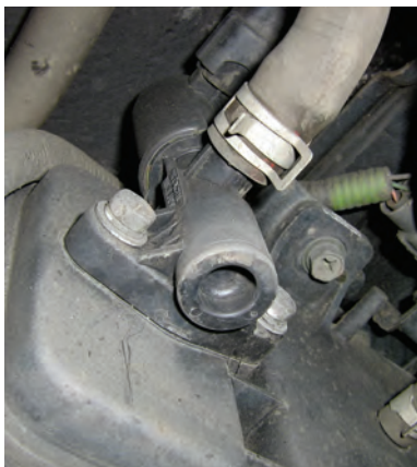
Figure 5 The canister vent valve is activated on during self-test.
