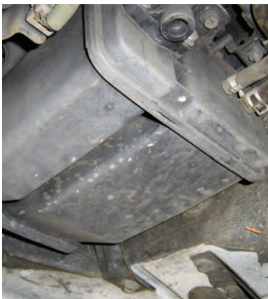
Figure 4 The canister stores and separates fuel vapors.
