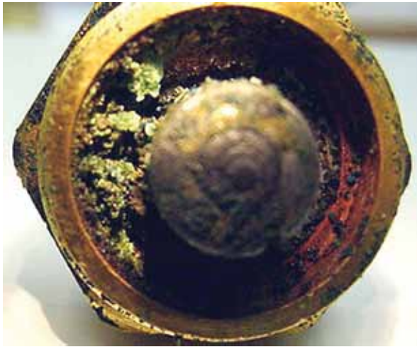
[Above] This recycling machine solenoid is plugged with A/C system sealant. Not good.
