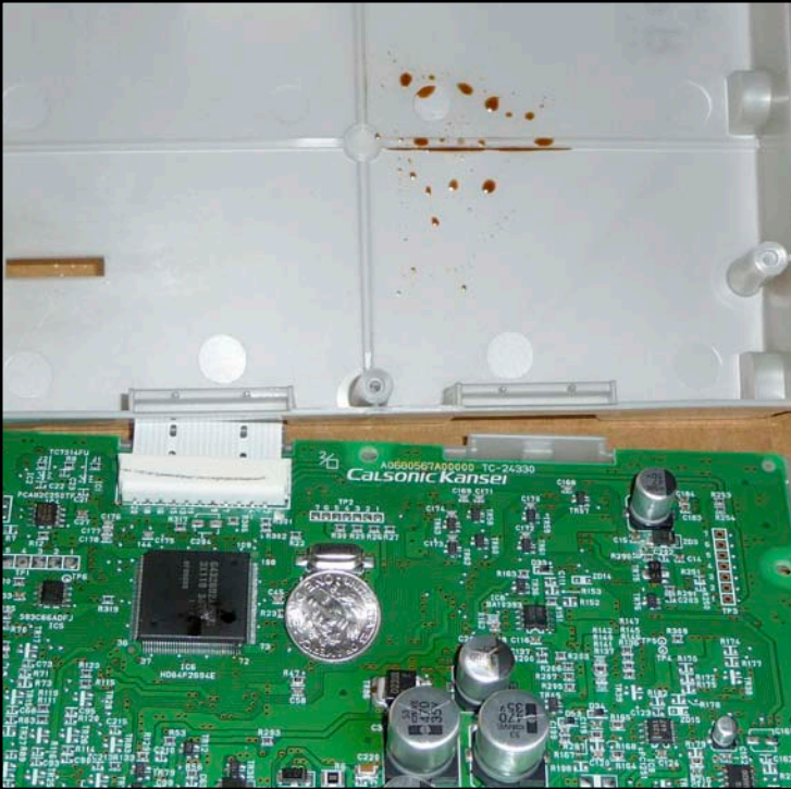
Figure 7 Left: brown residue of blown capacitor.
