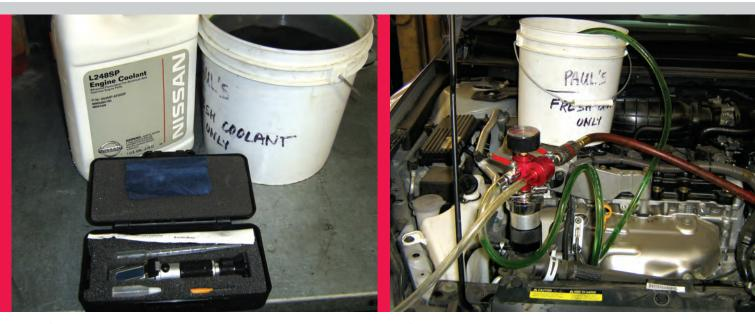
Mix coolant 50/50 then verify with a coolant refractometer or hydrometer.
