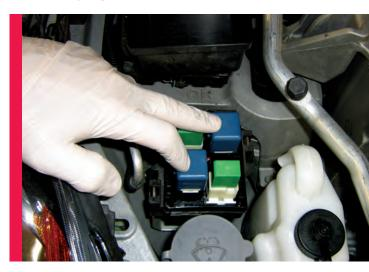
These are the ABS Pump Motor Relays.
