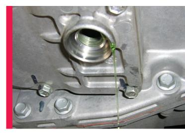
This is the inverter coolant drain in the transaxle. The other drain is on the inverter radiatior.
