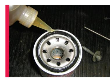
Always lubricate the oil filter gasket with clean motor oil so it won't become stuck in place. The "next guy" may be you!
