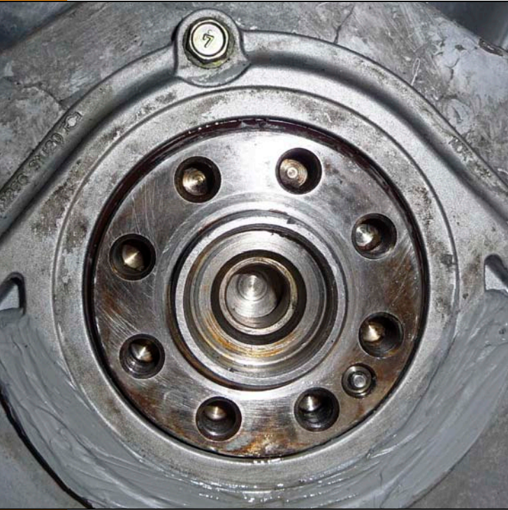
Figure 6 Above: Removed the flywheel to inspect where the dowel actually was located on the end of the crankshaft.
