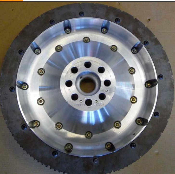
Figure 7 Below: flipped the flywheel over without losing the position the shop had originally installed.
