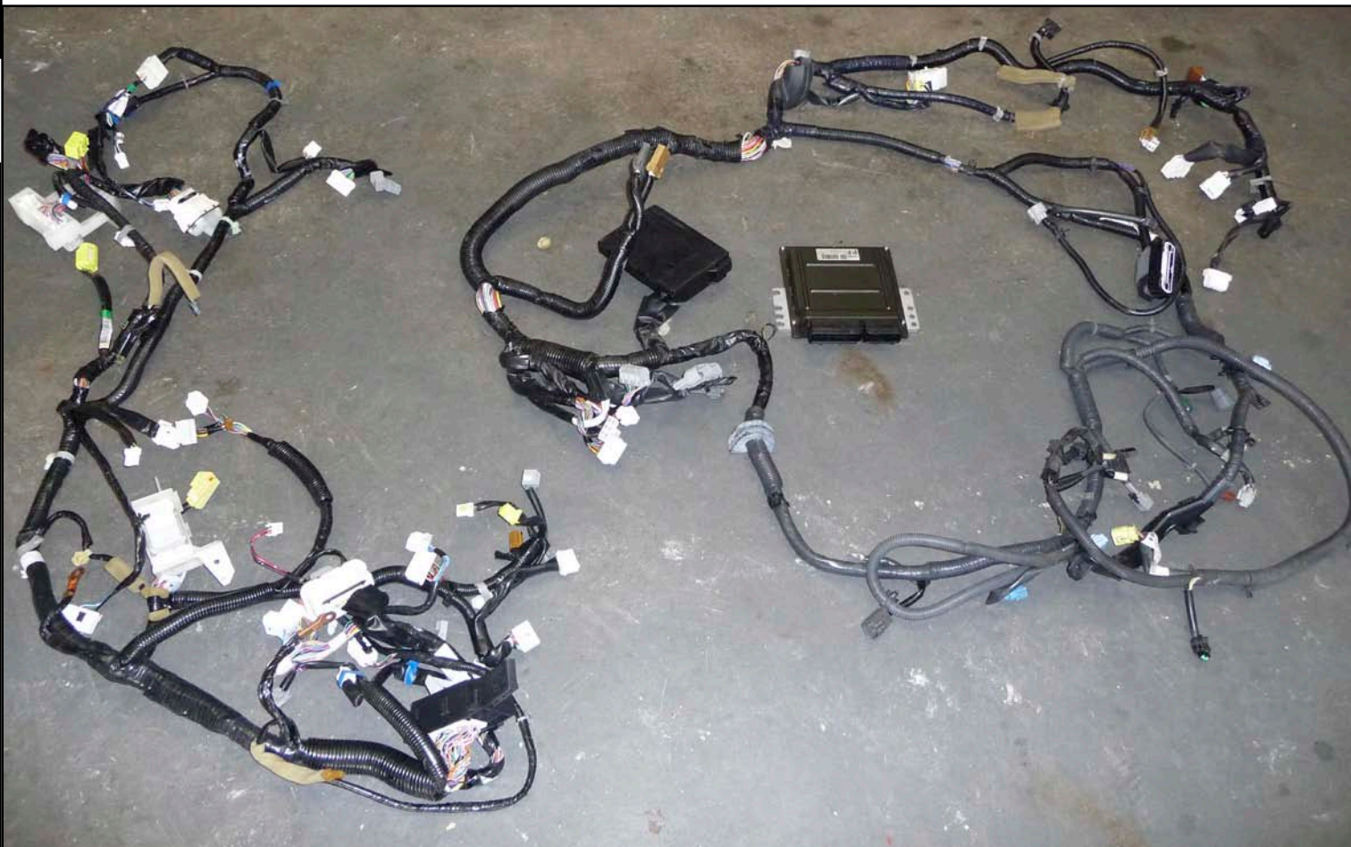
Figure 2: The entire Engine harness, dash harness and ECM were also replaced from the salvage vehicle.
