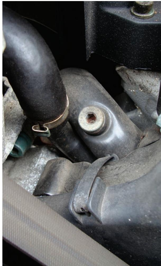
**While refilling the V6 cooling system, you should have the bleeder screws open to allow air to escape. This one is mounted on the cooling pipe next to the driver's side cylinder head, toward the front of the engine.**
