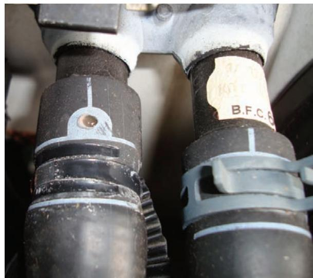
**Two high points in the system are the heater core hoses. The return hose has a hole that's normally blocked by the heater core pipe. To bleed the air out, remove the clamp and pull the hose off until air escapes and coolant starts to come out, then push the hose on and clamp it.**
