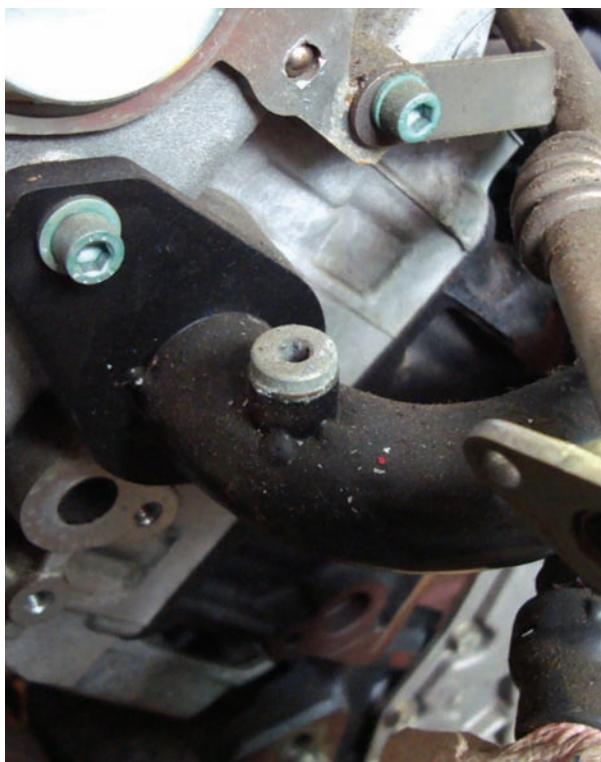
**A bleed screw that's harder to find is the one on the rear cooling pipe by the driver's side cylinder head. Without bleeding from this point, you may notice little to no heat in the cabin.**
