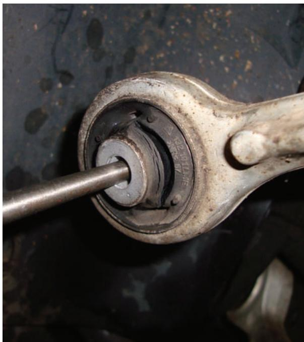
**Try twisting the bushing either attached or removed. If you can see tears like these of the upper link, this is definitely an issue that requires replacement, and OEM is the way to go.**
