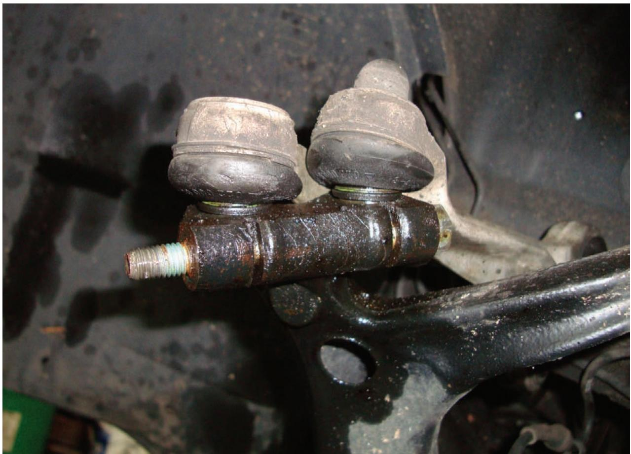
**This long bolt that mounts the upper ball joint to the spindle is probably the most difficult bolt to remove. Volkswagen does not recommend using heat on any suspension components. Use a penetrating fluid and work the bolt out.**
