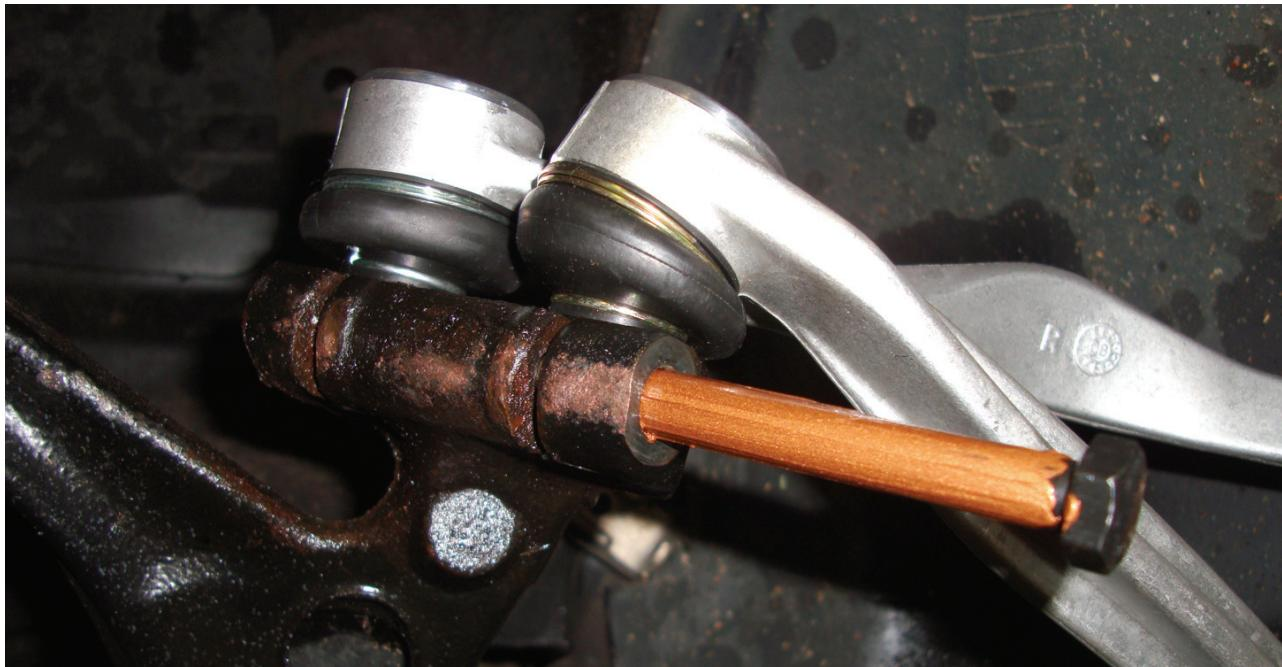
**While servicing these links, it is a good idea to provide some corrosion protection to the metal mating surfaces. This will make future service easier. Clean out the mounting bolts holes first with a wire brush.**
