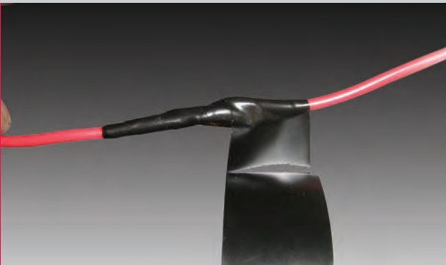
Wrap over the repair to an equidistant point on the other side of the repair, overlapping the tape by 50%.
