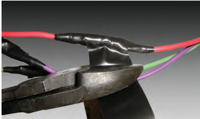
Cut the tape rather than pulling apart for neater appearance and better adhesion.
