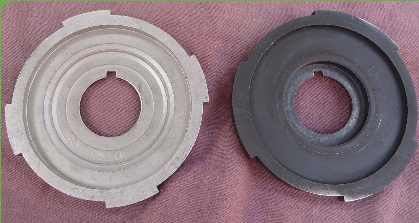
Figure 8: Both trigger wheels are configured to fit on the same crankshaft with no problem. The correct one had four triggers per revolution, instead of three.
