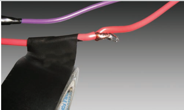
Begin wrapping to one side of the repair.
