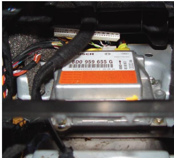
**The brain of the airbag system is the control unit, which is usually mounted underneath the dash panel, in front of the center console. You can access the connector and start checking wiring if damaged parts have been replaced, but you still have an airbag warning light on.**
