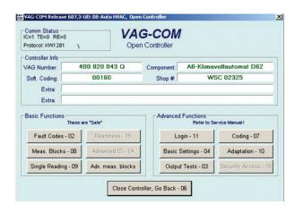
Here are your options once you have selected an address word. In 08, you can select "Basic Settings," enter "000," and the system will run through the initialization process. This should be performed after every mode door and temperature blend door replacement.
