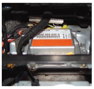
The brain of the airbag system is the control unit, which is usually mounted underneath the dash panel, in front of the center console. You can access the connector and start checking wiring if damaged parts have been replaced, but you still have an airbag warning light on.
