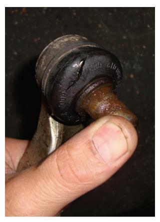
While examining suspension components, check for torn boots on the ball joints, which will allow dirt to enter the socket and accelerate the wear that creates noises and suspension vibration.
