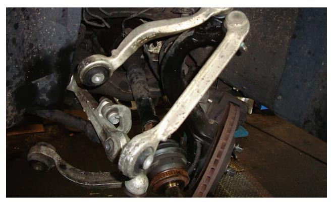
Aluminum links will eventually wear out on high-mileage vehicles. Finding out which link is the problem will require some diagnosis and testing. Using OEM Volkswagen parts will ensure long service.
