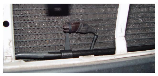
This is an ambient air temperature sensor found on an automatic climate control system, and is not to be confused with the ambient air temperature switch found on manual system. This sensor will only flag a code and affect temperature control. It will not suspend compressor operation.
