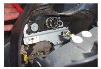
Removing an airbag sometimes involves that you have a "feel" for the vehicle. While placing a small screwdriver down a blind hole, you need to feel for the spring and pry upwards moving the spring in. This releases the pin for airbag removal.
