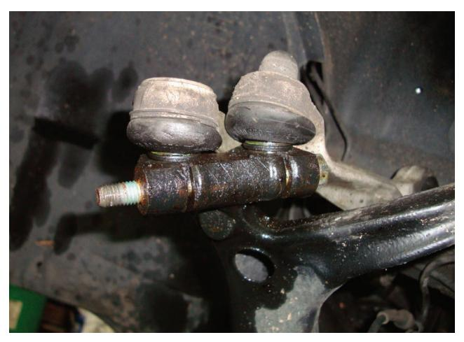
This long bolt that mounts the upper ball joint to the spindle is probably the most difficult bolt to remove. Volkswagen does not recommend using heat on any suspension components. Use a penetrating fluid and work the bolt out.
