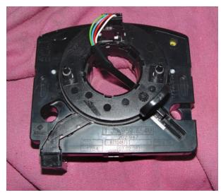
The clock spring maintains the electrical connection between the airbag control unit and steering wheel-mounted airbag no matter what the position of the steering wheel. When a deployment has occurred, it must be replaced with the airbag.
