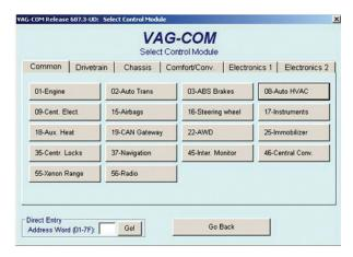
As you can see, there are many "address words" for all of the possible self-diagnostic systems on the vehicle. Select address word 08 – HVAC and you can talk to an automatic climate control system (not a manual system).
