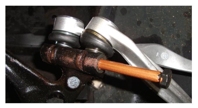
While servicing these links, it is a good idea to provide some corrosion protection to the metal mating surfaces. This will make future service easier. Clean out the mounting bolts holes first with a wire brush.
