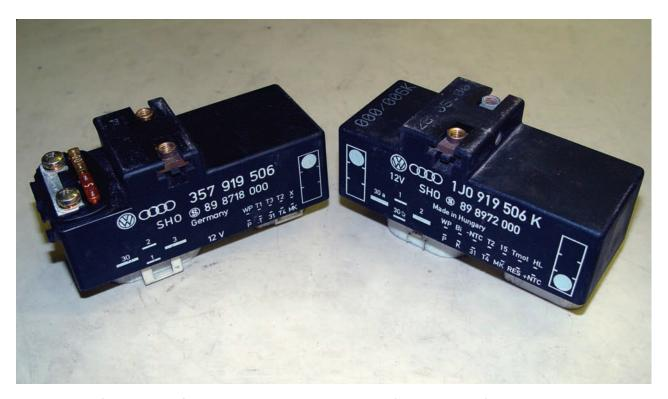
On the side of the cooling fan control unit, the pins are identified with their functions. You may be able to use them for testing once you learn what they are. Note that both strip and ATC fuses can be blown and prevent AC and cooling fan operation.
