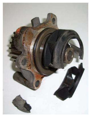
Here's something that can happen inside an engine that you can't see. The impeller has separated from the shaft and is no longer spinning. An outside view doesn't indicate a failure since the water pump bearing is intact. Watch coolant temperature at the rear of the cylinder head and check to see if it is building up too slowly, which means low circulation.
