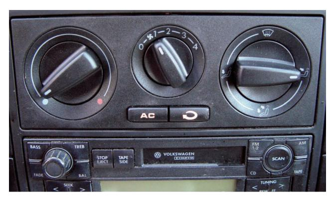
The famous three dials of the Volkswagen HVAC system tell us when the AC button is pushed and the blower motor is turned on. The switch provides voltage to pin #8 on the cooling fan control unit indicating that AC has been requested.
