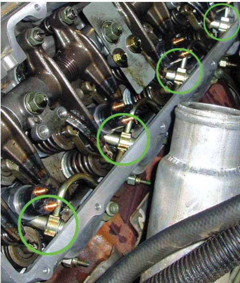
Figure 1: The biggest and most public issue with the motor was its tendency to crack the fuel injectors here.
