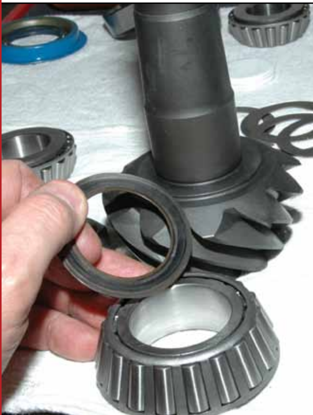
Depth shim under rear pinion bearing.
