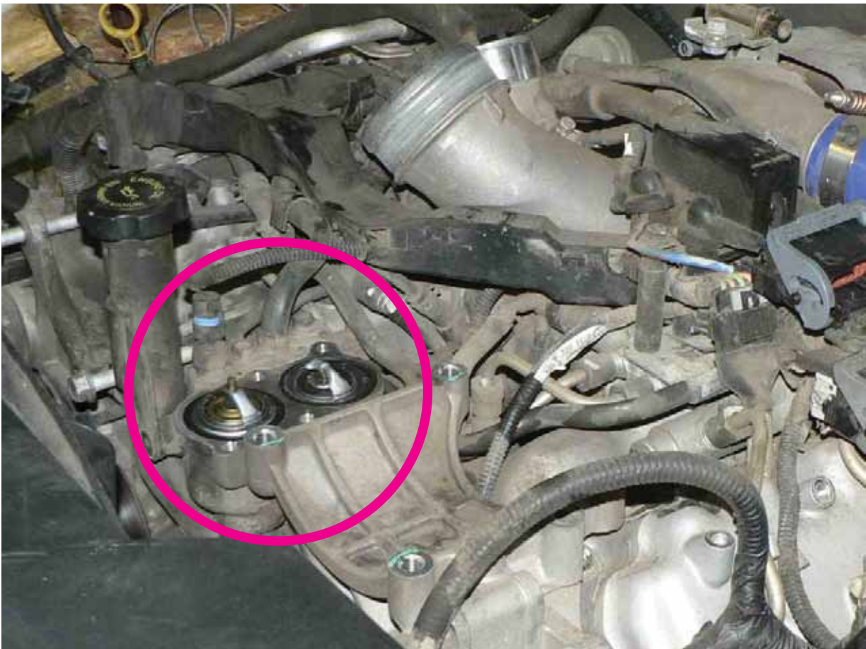
Figure 6: Lots of stuff in the way even after the accessories are off the front. Note the dual thermostats.
