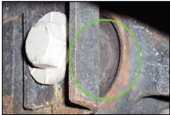
Figure 20: This lower control arm bushing is cracked.
