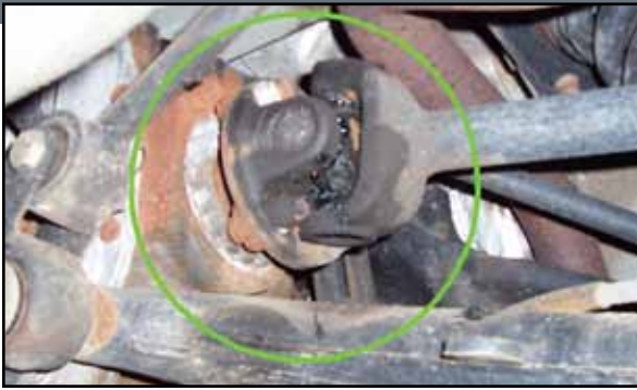
[Above] Figure 23: The rear camber adjustment shim is sandwiched between the differential and half-shaft flanges.
