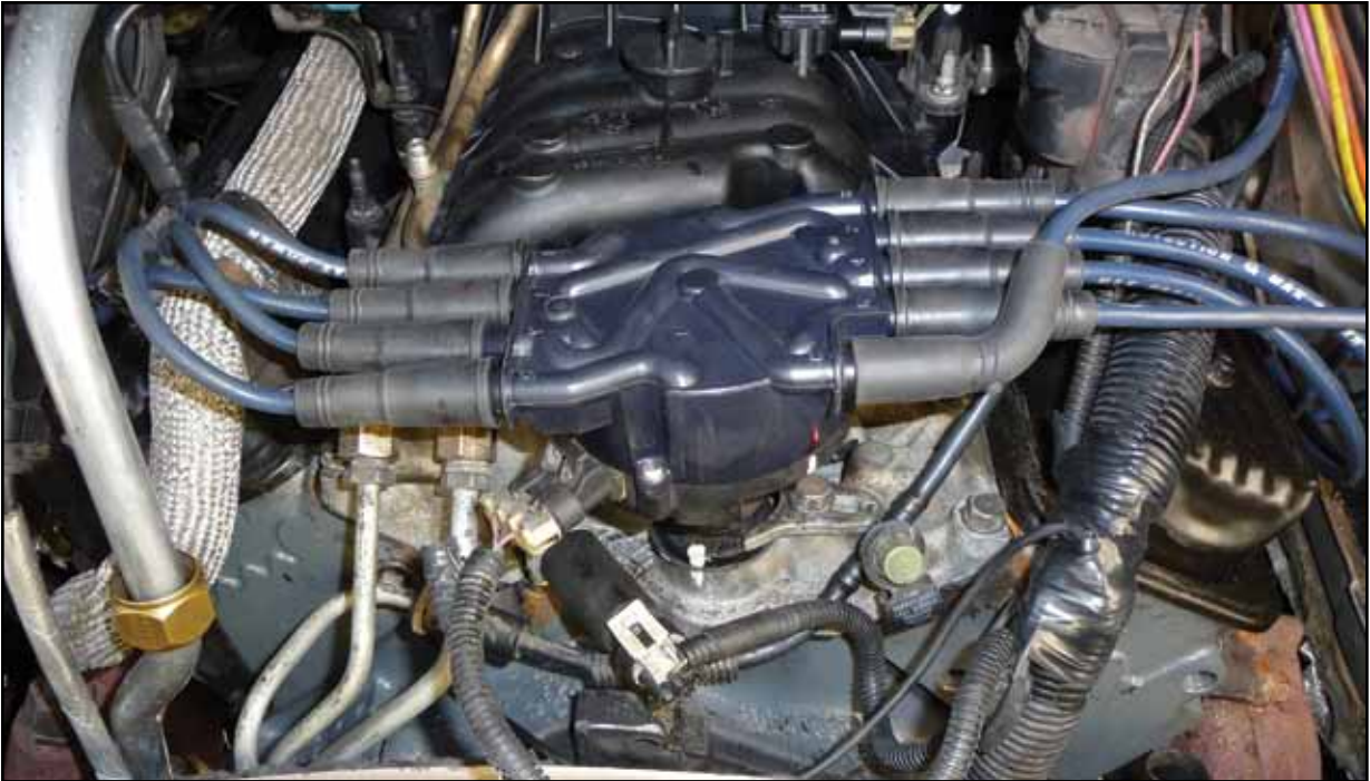
Figure 3: The distributor housing base was marked with the intake manifold to guarantee a correct orientation of the distributor housing location.
