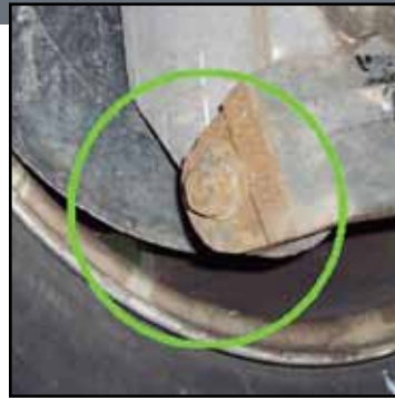
[Above] Figure 23: The rear camber adjustment shim is sandwiched between the differential and half-shaft flanges.
