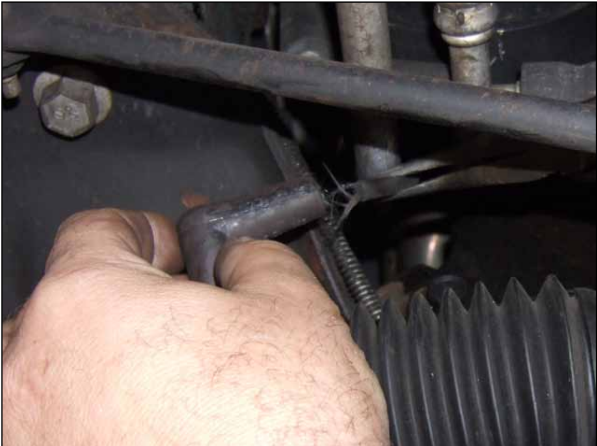
Figure 8: We lifted the vehicle and removed the #6 spark plug wire and the boot actually separated itself from the wire.
