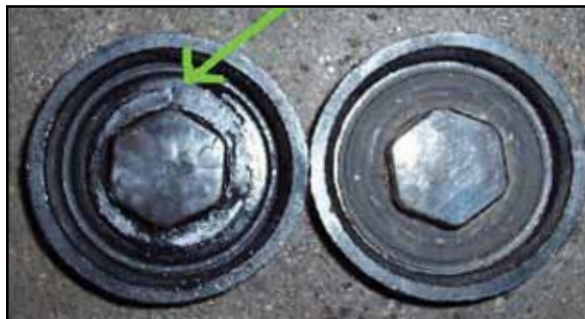
Figure 16: This seal retainer is starting to crack.
