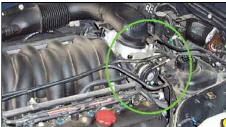
Figure 9: On the AJ-27 engine, the throttle body assembly lacks the cruise control chamber.
