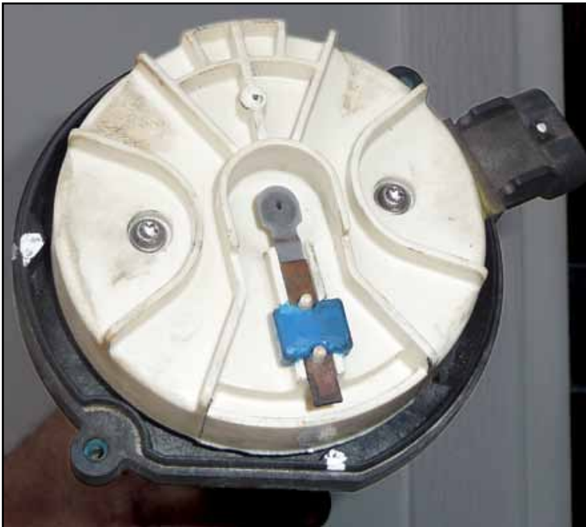
Figure 4: the same distributor being used for both the 4.3L and 5.0L and how there were two different positions to index the rotor to the distributor housing.
