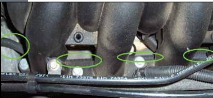
Figure 19: The part-load vacuum hose is routed beneath the intake runners.
