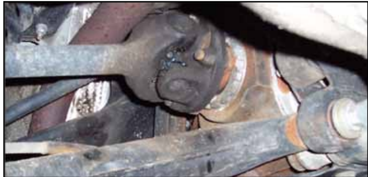
Figure 21: All four rear half-shaft u-joints are greaseable, yet often overlooked.
