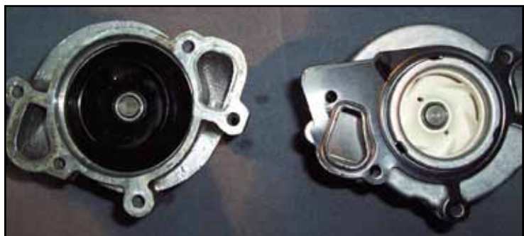
Figure 17: The white impeller distinguishes the newer style pump.
