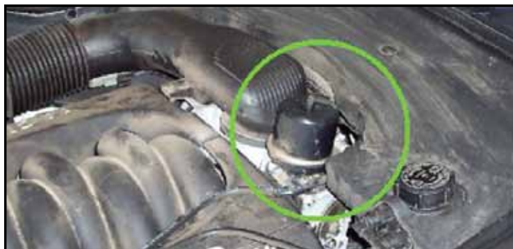
Figure 8: The AJ-26 engine has the cruise control chamber on top of the throttle body assembly
