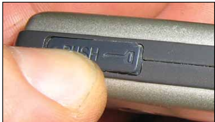
The Smart Key insert can be removed when the release button/slider is actuated.
