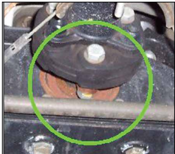
Figure 22: The differential pinion seal is prone to leaking.
