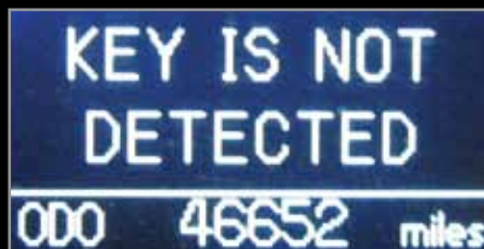
Wrong key message for Camry HV.
