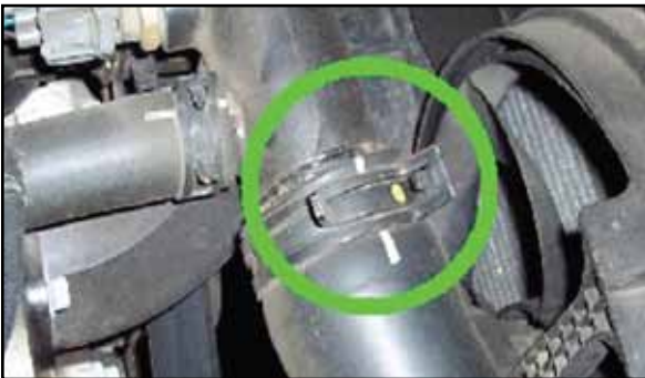
Figure 13: This hose is starting to slip as well.
