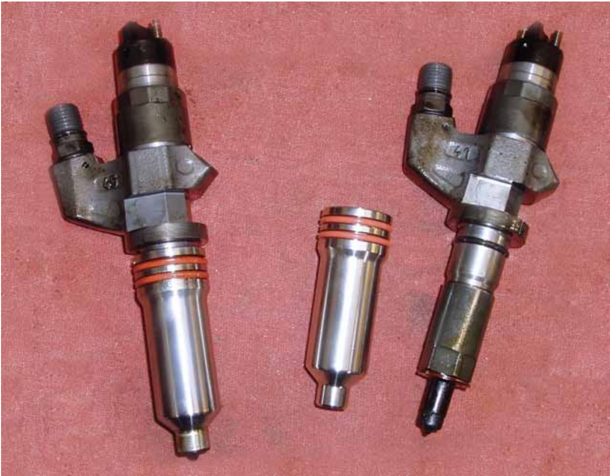
Figure 2: LB7 injectors sit in a coolant-cooled sleeve that is pressed into the hole in the cylinder head with GM special tool J 45910.
