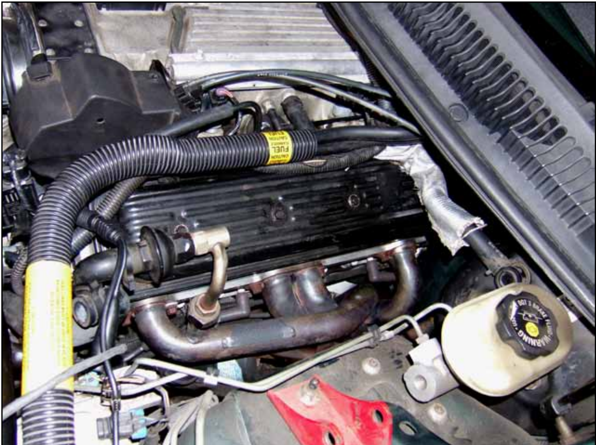
Figure 7: Someone had changed the stock exhaust and installed header pipes.
