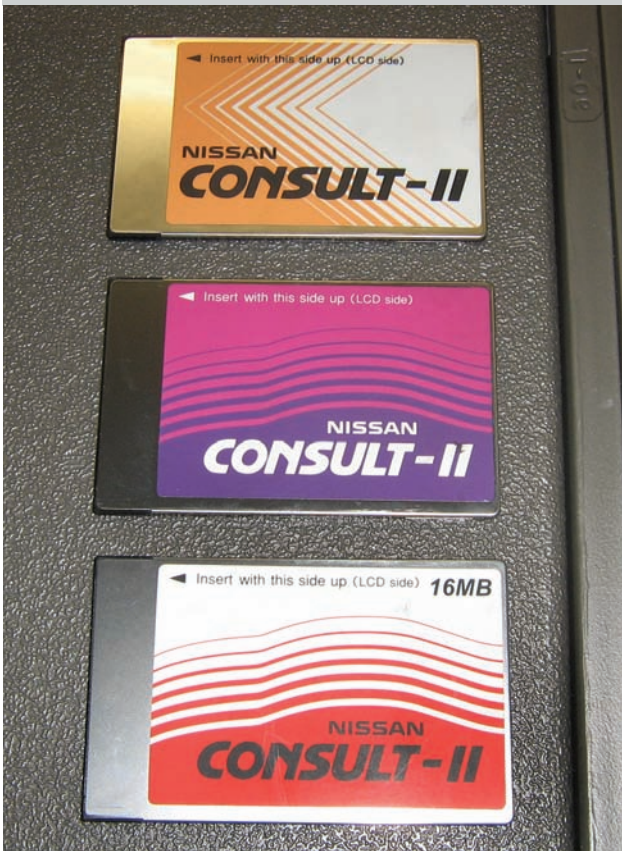
Top to bottom: Programming card (orange), NATS card (purple), Diagnosis card (red).
