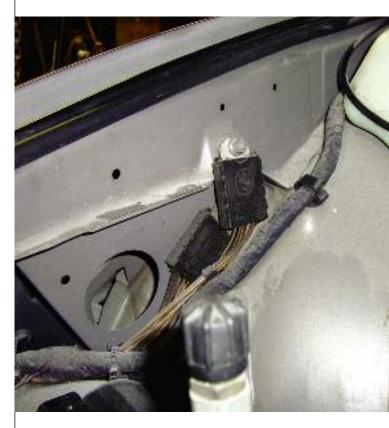
On 2004 and later 5 Series, the entire front clip is aluminum, including the firewall. The unit is bonded and riveted to the body. Be sure to add the ground strap to prevent any electrical problem. Look through you archives of TechDrive for a previous article on grounds.
