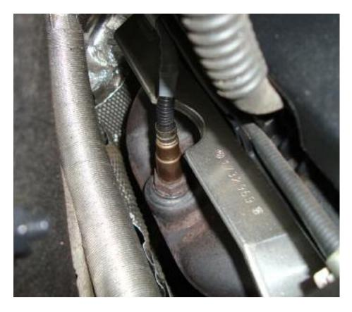
No longer are air/fuel ratio sensors mounted in the down pipe. They need over 750 deg. C. to function properly. Also notice how they are mounted straight up. This prevents condensation from getting trapped in the sensor, and it also makes service much easier.
