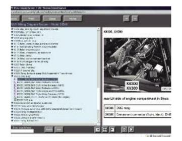
By selecting one of the green links inside the wiring diagram, you will be directed to a pull-down menu in the navigation bar. After selecting the particular variant, you will see the component location of the link you selected. This can make finding fuses, relays and splices easy.
