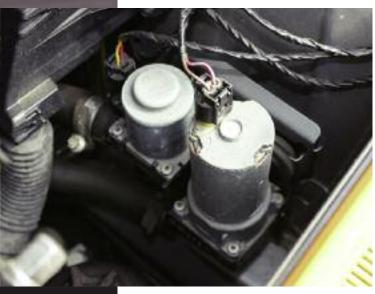
This single heater control valve is mounted behind the auxiliary coolant pump. It determines how much coolant makes it to the heater core, and the auxiliary coolant pump assists flow when heating demand is high.
