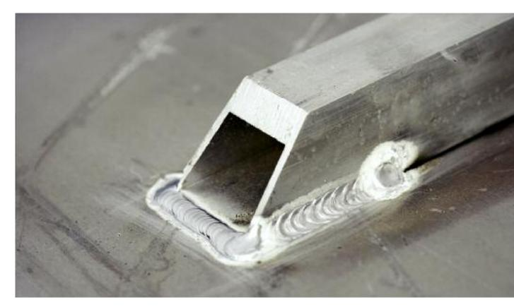
Although currently BMW does not recommend straightening aluminum, some day it may approve aluminum-to-aluminum welding. Be prepared to tool up with an inverter-type welder, which pulses current across the welding tip to keep metal temperatures down.
