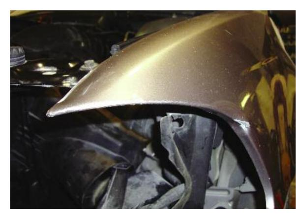
Although to repair this damage is time-consuming relative to the surface area involved, these aluminum panels should be repaired. The general rule with aluminum is to start from the outer most portion of the damage and work inward toward the middle.
