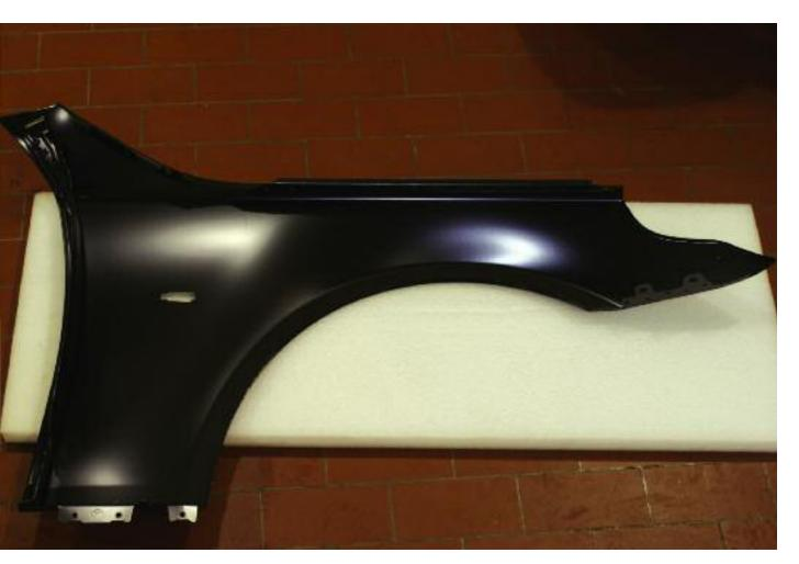
Aluminum panels purchased from your BMW parts supplier come already primed. After cleaning, they are ready to paint with BMW Colorsystems. A typical fender replacement may be more profitable than straightening.
