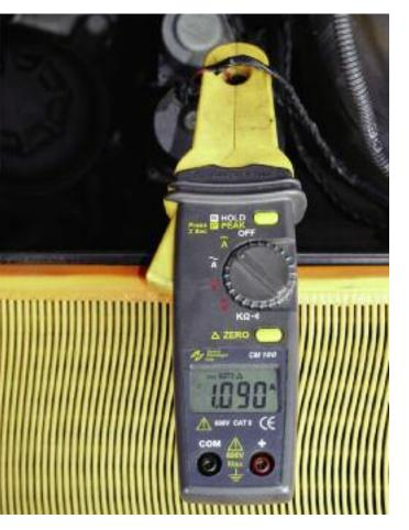
With the temperature set above 80 deg. F., you should see the auxiliary coolant pump activated. It should draw about one amp at full speed, but it's normal for a cold engine to increase that draw to about 1.3 amps.
