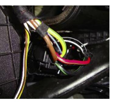
The final stage unit is usually located behind the glove box. The yellow wire with a green tracer is the power supply from the heater relay, the brown wire is ground, and the red wire with a green tracer is the power supply. The black wire with a green tracer is the ground supply to the blower motor, and, finally, the blue wire with a red tracer is the control wire from the IHKR or IHKA control units.
