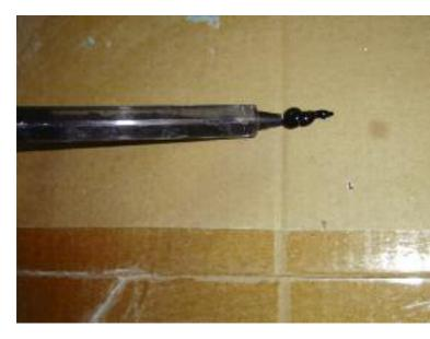
As you can see, the bonding agent is not evenly dispersed in the mixing tube. This chemical bond will not dry or adhere properly. Equalize the mix by squeezing out an inch of material before and after installing the mixture tube. Get better performance from a cleaner engine with BMW Group Fuel System Cleaner Plus.
