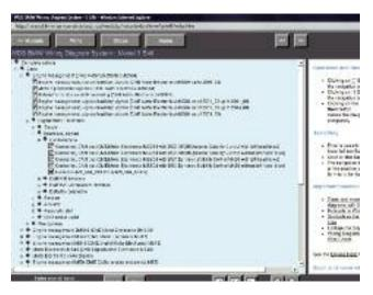
The first critical step is selecting the correct wiring diagram. You will need to choose among all the different variants of the vehicle. This can include production dates, options (ASC or DSC, for example), body style, left/right hand drive, version level, etc.
