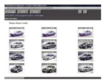
Once WDS is started and the plug-in is installed, you will see the main navigation screen. Select "Complete Vehicle" and pull-down menus will start to appear just as they do in Windows Explorer on your PC.
