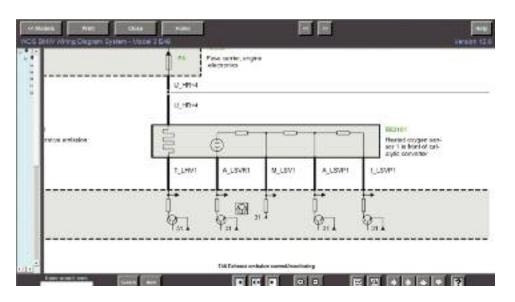
Through www.bmwtechinfo.com you can view the wiring of the air/fuel ratio sensor. Notice that there are six wires in the diagram, but only five on the sensor itself. That's because you're seeing the harness side of the connector.
