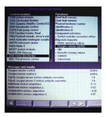
When using your scan tool, you may be tempted to watch the air/fuel ratio sensor voltage and make a determination from that. Here you see that both AFR sensors are reading 1.6 volts after opening the throttle, which you will not see on any wire at the sensor. This show activity but not much else.
