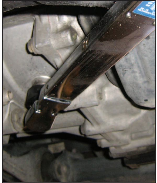
Install the inverter drain plug and torque it to 29 ft/lb.
