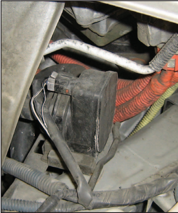
5. Once the headlight is out of the way, the pump is easy to access.
