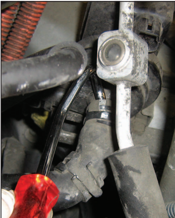
If you are planning to reuse the hoses, use a hose pick to separate the hoses from the inlet and outlet.
