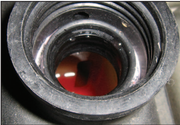
If the coolant is still or barely moving, there's a problem.
