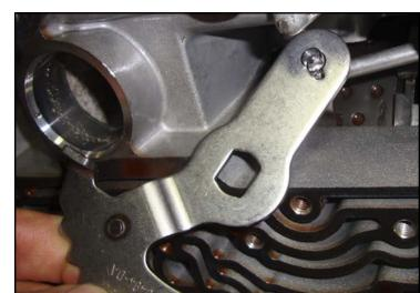
dropping the valve body, you need to know that there's a spring between the valve body and the case of the transmission.
