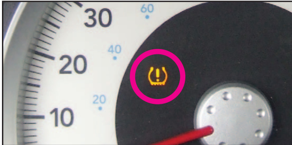
Figure 8: Dodge Durango with complaint of Tire Pressure Monitor light on.
