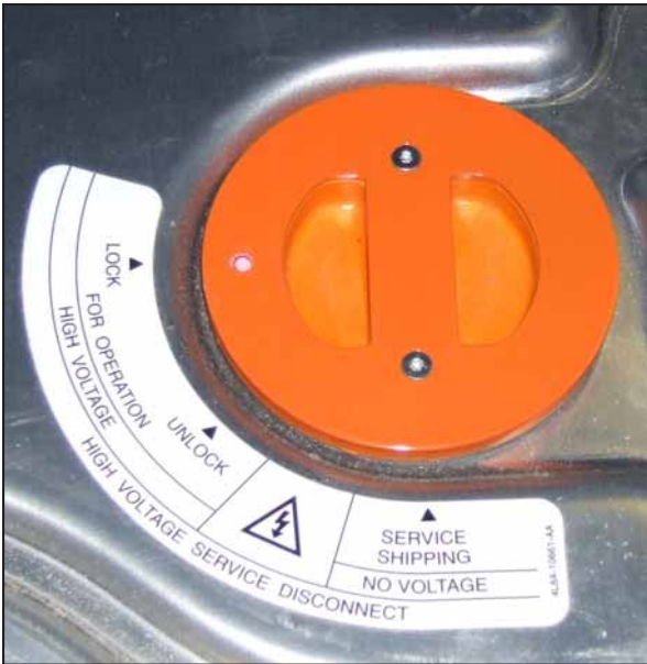
Figure 5: A closer view shows that there are three possible positions the plug can be installed in (Lock, Unlock or Service Shipping)
