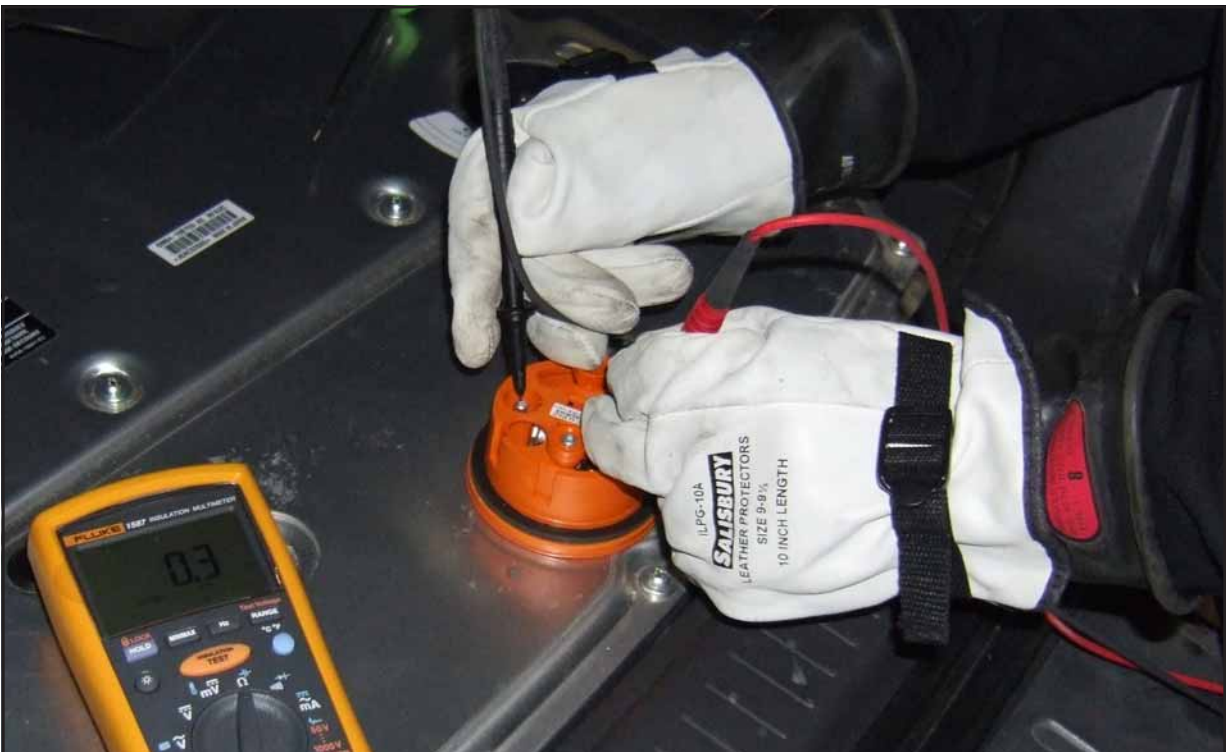
Figure 6: I removed the plug and used my special CAT5 Hybrid-rated Fluke 1587 meter to test the fuse within the safety plug.
