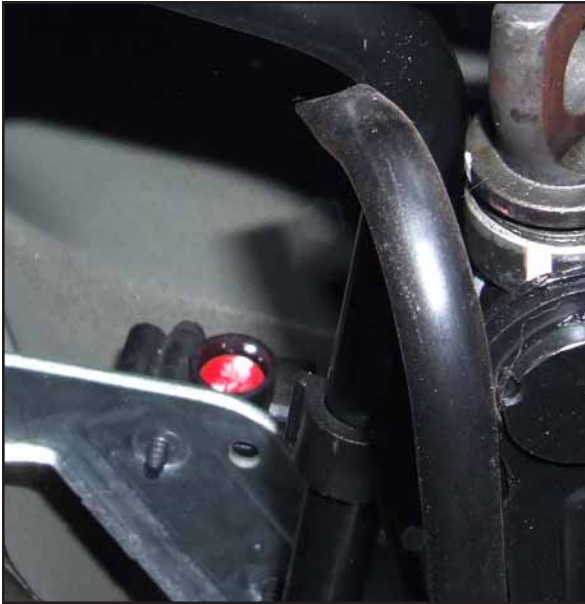
Figure 7: Also located in the rear compartment in the right rear quarter panel is a hybrid inertia switch.
