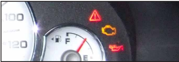
Figure 2: An attempt to start the Escape and it would not do anything. The “Red Triangle of Death” was lit up on the dash indicating a serious hybrid problem.
