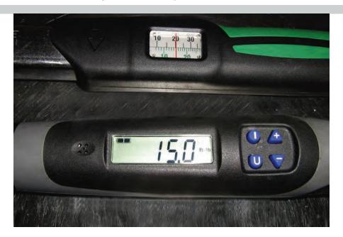
Select a torque wrench that can accurately measure 14-22 ft. lbs.
