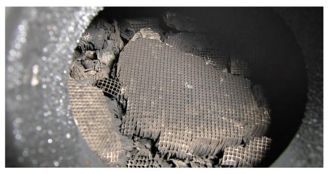
This converter damage was caused by a chronic misfire.
