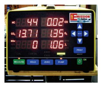
An exhaust analyzer with a Lambda display should be used to confirm proper air fuel ratio.
