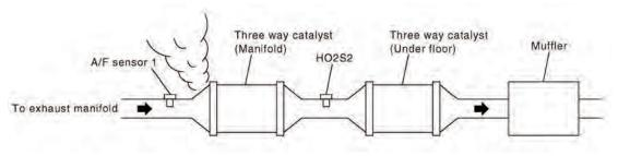
An exhaust leak will reduce the converter's efficiency.
