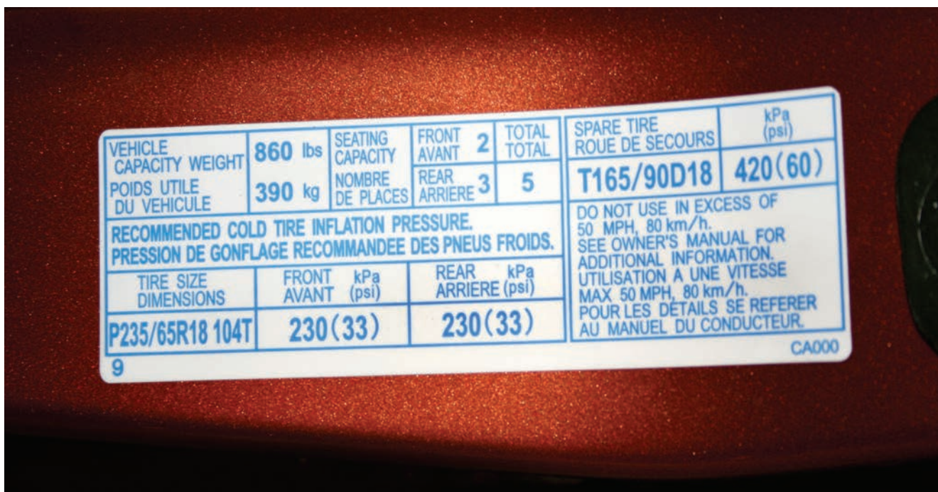
The Tire and Loading Information placard displays the proper tire inflation levels.
