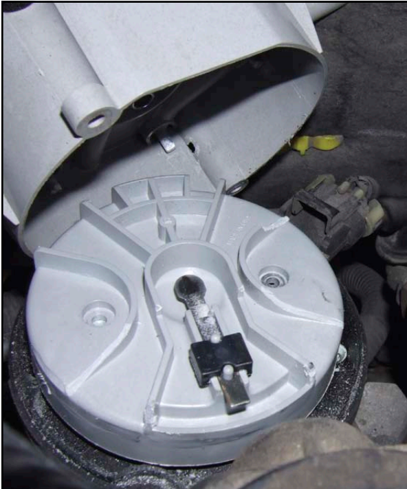
Figure 5: The distributor rotor was no longer secured to the distributor shaft because both screws were missing.
