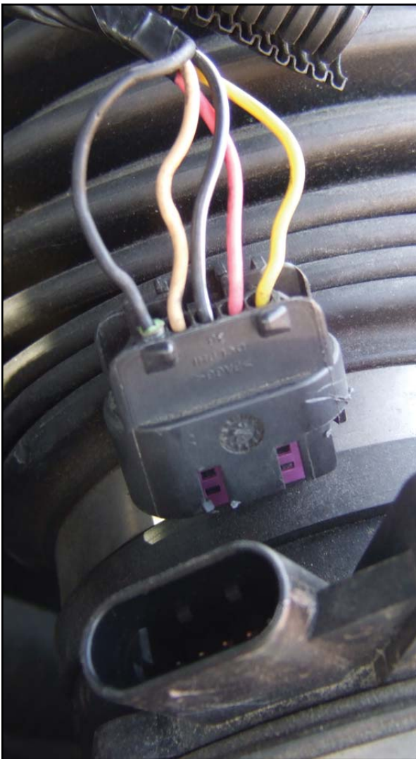
Figure 6: The IAT reference ground had backed out of the connector.
