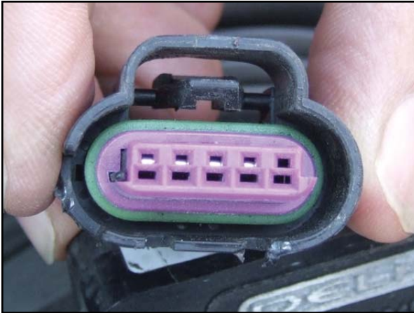
Figure 5: After pulling the connector, only four pins show at the end of the connector.
