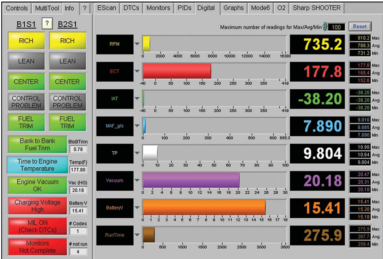
Figure 3: To verify the IAT failure, I selected the IAT parameter in digital format and I could see the -38 deg. F.
