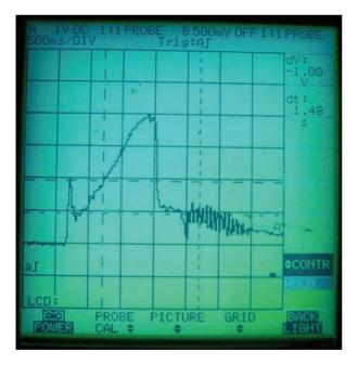
Here is a scope pattern of a 1.8L turbo MAF. The first spike to three volts is the snap of the throttle. The second spike up to over four volts is when the engine revs to 4,000 rpm. This MAF is not creating any fuel trim problems.
