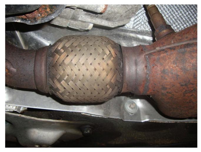
When testing O2 sensors, you need to make sure the exhaust system is sealed. Here we have a leaking flex joint. This allows fresh air into the exhaust, which affects the O2 sensor signal. Use a smoke machine to check for leaks in the exhaust system.
