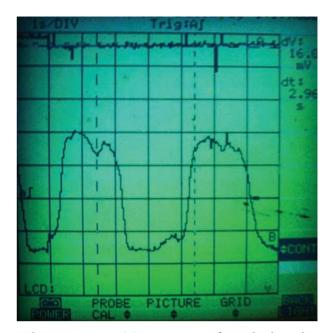
When testing an O2 sensor waveform, look at the signal voltage's highest and lowest points. Also look at the total number of switches over time. You should see about one full switch per second. Volkswagen OEM O2 sensors will ensure performance to Volkswagen standards.
