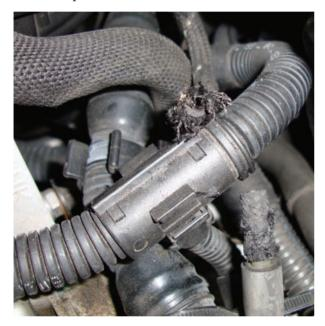
Never underestimate the visual inspection. Here we have a broken vacuum hose. This vacuum leak will lean out the mixture to a point of setting a code. Adding smoke to the intake manifold will help locate hard-to-find leaks.
