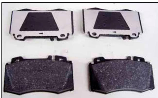
*The OEM pads provided by your Mercedes-Benz dealer have chamfered friction material to help avoid brake noise. The shim on the back reduces brake pad vibration, which is what causes squeal.*
