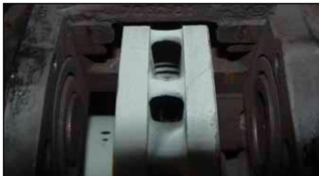
*Look at the surfaces where the pads slide in the caliper. These areas need to be free of brake dust and corrosion to allow the pads to slide back and forth. If the surfaces are clean, you should not need any lubricant.*
