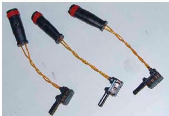
*While ordering brake pads and rotors, don't forget the brake pad wear sensors. You should replace them even if the old ones are not worn out. Be careful not to route the wires so that they bear against any moving parts.*
