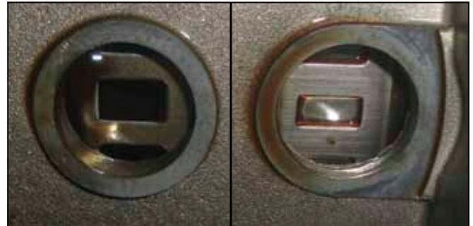
*Above the valve body are speed sensors N2 and N3. They fit into the lower part of the case and indicate the speed of the clutch basket tone wheel. This is how the control unit determines slippage. Make sure you do not have any speed sensor problems before trusting scan data.*
