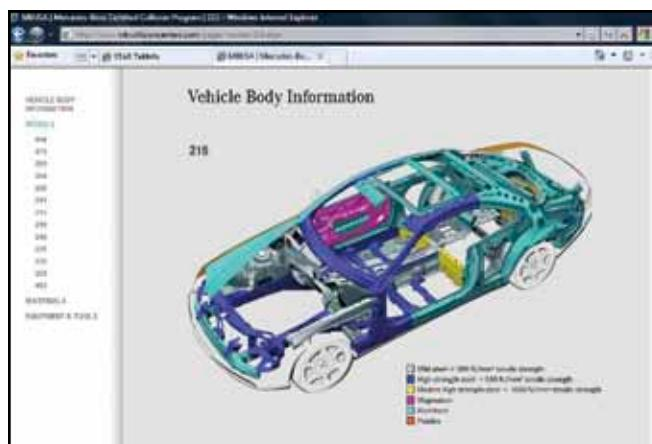
*Being a Mercedes-Benz Collision Center gets you access to the website. This information is vital to making the proper repair. Here you can see the different materials used in a 215 chassis.*
