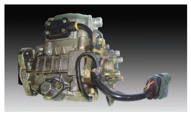
Looking at the pump harness, you will see that one plug supplies all of the electrical components. The lower harness goes to the cold start injector. The upper harness goes to the fuel shut-off solenoid and the quantity adjuster (left). The position sensor and fuel temperature sensor are mounted inside the pump.
