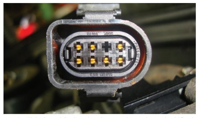
Notice the gold-plated terminals for a better electrical connection. The terminals are numbered differently from what you might assume. Here, terminal 1 is in the lower left hand corner, and terminal 2 is in the upper left hand corner -- they power and ground the motor.
