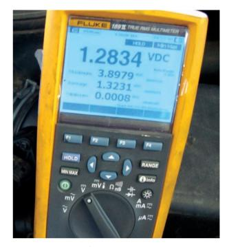
With a new MAF from your Volkswagen dealer's parts department you see a difference in peak signal voltage after a throttle snap almost reaching 3.9 volts. This is good for the 2.0 liter engine. Other engines may have different specs.
