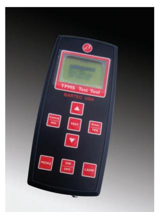
Aftermarket tools are available for testing TPMS sensors. You'll need to activate the sensor and set the tool to pick up a 315MHz signal. The display will let you know that the sensor is transmitting.
