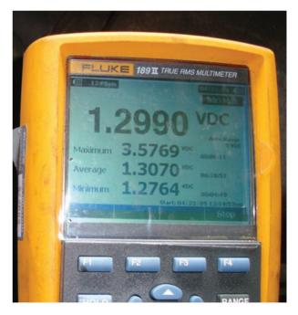
Look at the voltage specs on this 2.0 liter engine. The average and current signal voltage is around 1.3 volts. Look at the maximum voltage. It is only 3.5 volts after a throttle snap. If everything else is okay, you may need to replace it with an OEM sensor from your Volkswagen parts supplier.
