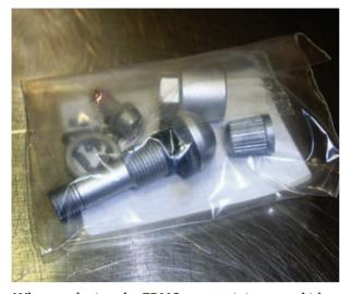
When replacing the TPMS sensor, it is a good idea to replace the valve stem assembly. OEM level quality parts are available from an authorized Volkswagen dealer.
