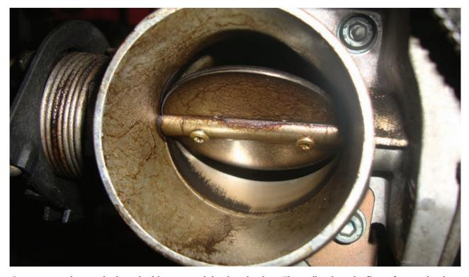
Over time, carbon and oil can build up around the throttle plate. This will reduce the flow of air and reduce idle speed. The PCM can compensate by opening the throttle more. When the idle adaptation is lost, low idle and decel stalls may result.
