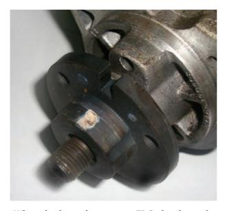
When checking alignment at TDC, the slot in the flange is at the 12 o'clock position relative to the pump. Here is where you put the special tool through the pulley into the hole pictured here in the injection pump. Using a genuine Volkswagen timing belt will help ensure both proper valve and injection timing, and long life.
