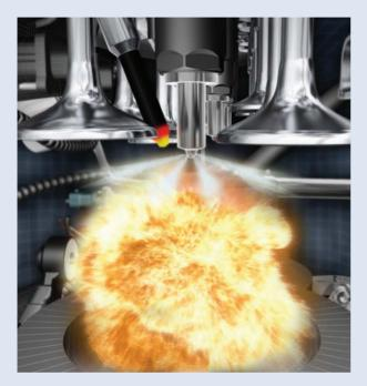
Direct injection increases fuel efficiency by up to 20% over the use of pre-combustion chambers.
