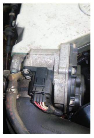
If you see a cable on the throttle body, you'll know this is a ME5 system. The electronic throttle only controls idle speed and low rpm functions. The throttle will have to be re-adapted if you get a code P1580 or P1582.
