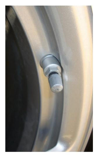
If you want to know if a vehicle has TPMS, look at the valve stem. If it has a silver retaining nut, it has the system. Set tire pressures to specs when the tires are cold.
