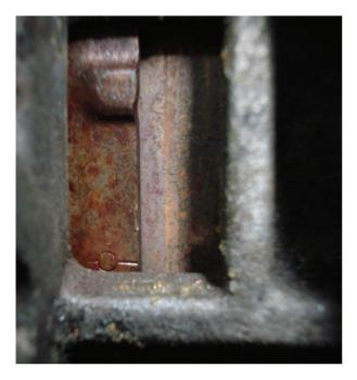
When checking basic injector pump timing, be sure the crankshaft is at TDC. Look through the opening in the bellhousing and you should see an "0" mark. Line up the mark with the lower edge of the opening and check the pump timing.
