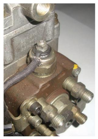
The fuel shut-off solenoid has a single wire to provide power. The body of the unit is the ground path. This solenoid is activated whenever the key is turned on. An anti-theft situation will turn off the solenoid, so monitor anti-theft data usually found in the instrument cluster, or immobilizer unit.
