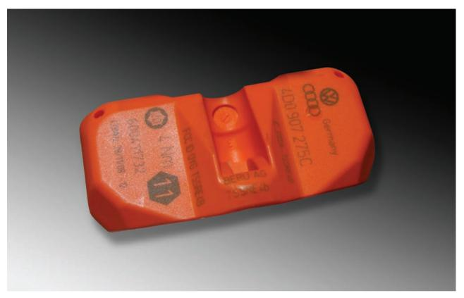
Here's the replacement sensor. It should last 10 years, but driving with a slow leak will constantly trigger the sensor to transmit the RF signal. This shortens battery life.
