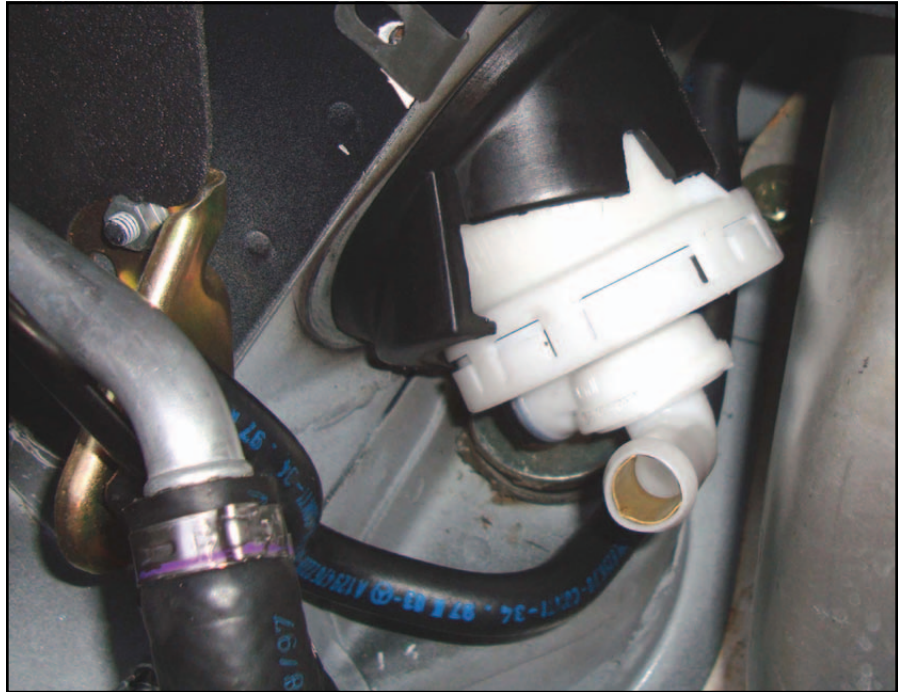
The vent cut-off solenoid normally allows air into the canister, but can be closed for a leak diagnosis. Contaminants can get into the solenoid and cause it to stick open or closed. This is why it is tucked away in the body of this '98 129 chassis.
