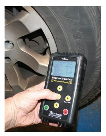
Activating TPMS sensors is quick and easy with the Signal Tech II.
