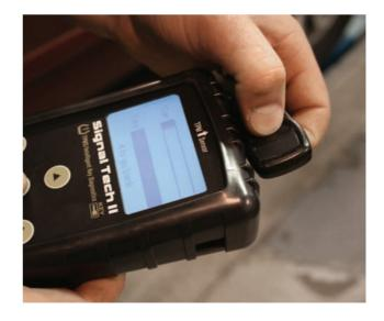
The Signal Tech II can also be used for checking RKE key fob signal strength.
