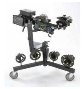
Everything needed to cut rotors on the vehicle is stored with the lathe.
