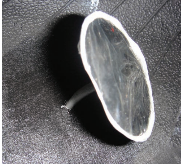
Insert the patch stem into the cleaned and cemented injury channel.
