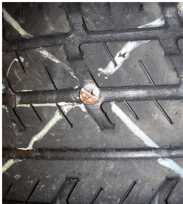
Mark the source of the leak before removing the tire from the rim. Some injuries can be hard to find again once the tire has been removed and there is no way to add air.
