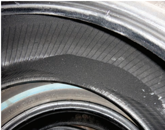
Rubber powder is a sign of tire damage.
