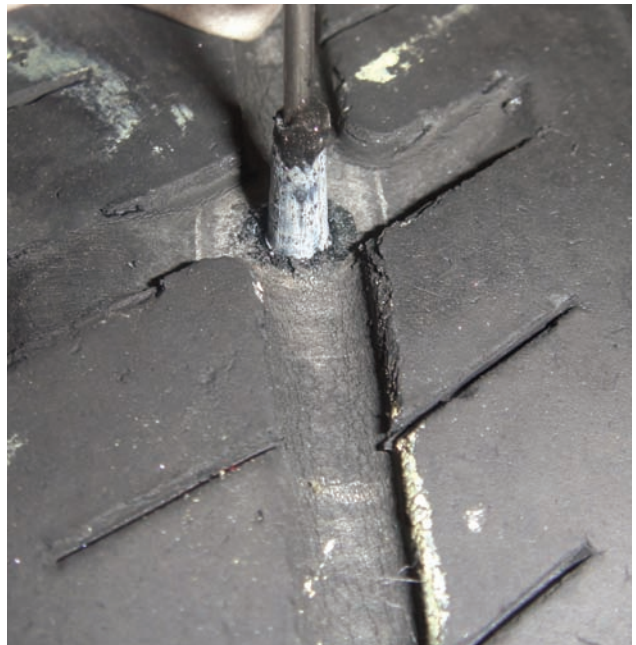
Once the stem is through, pull it from the tread side. This is easier than trying to push it through because the stem will tend to get thinner when it is pulled and thicker when pushed.
