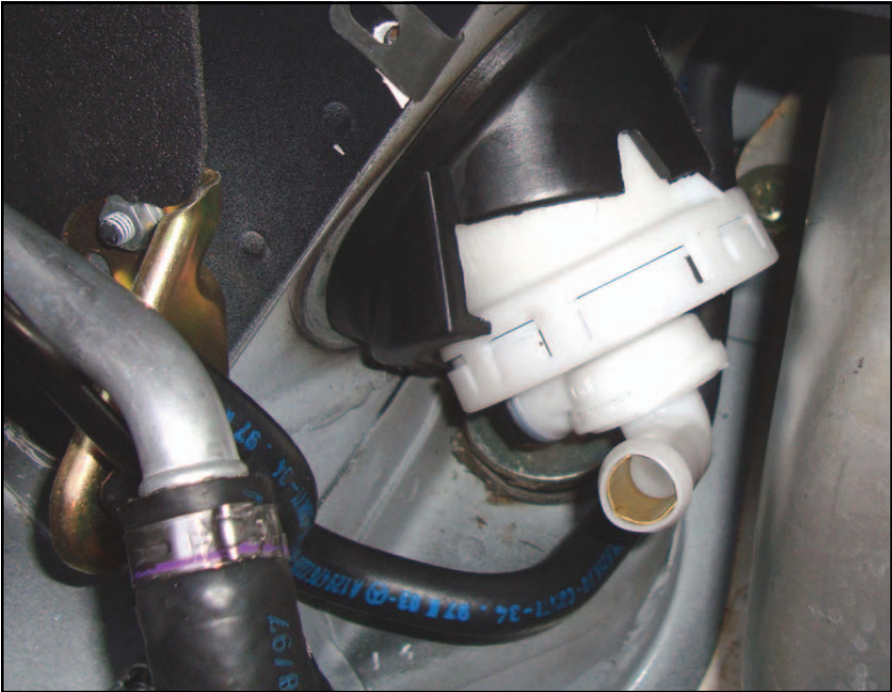
The vent cut-off solenoid normally allows air into the canister, but can be closed for a leak diagnosis. Contaminants can get into the solenoid and cause it to stick open or closed. This is why it is tucked away in the body of this '98 I 29 chassis.
