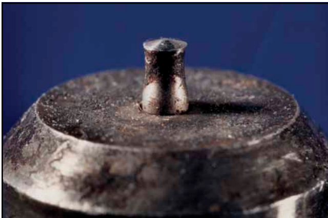
The deposits that form on a fuel injector's tip will distort the spray pattern.
