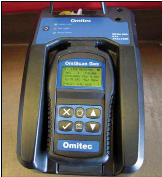
The handset of this 5-gas exhaust gas analyzer can be used in a wireless mode. The gas bench can be placed in the vehicle's trunk during a road test and you can still look at the readings.
