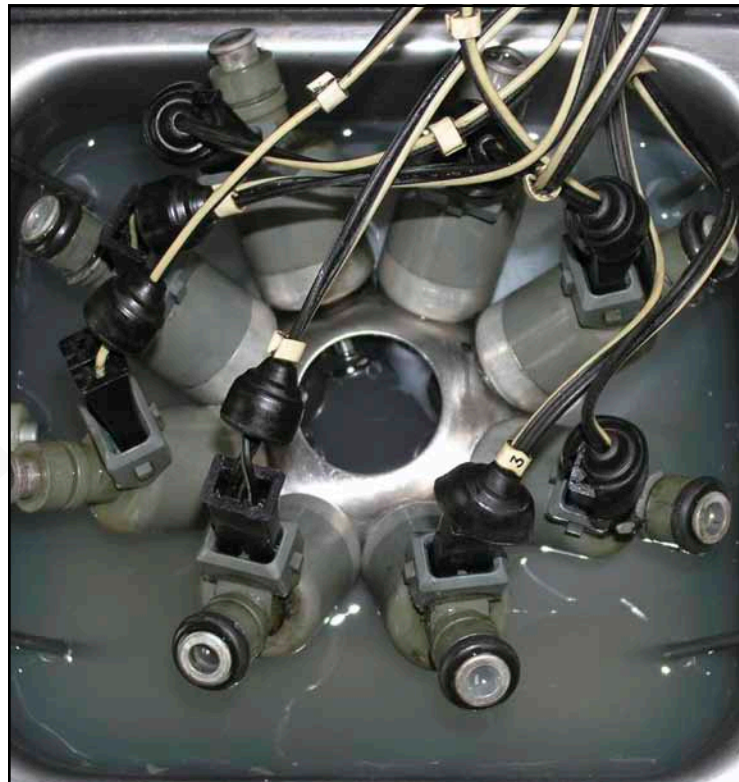
Fuel injectors being cleaned in an ultrasonic bath.
