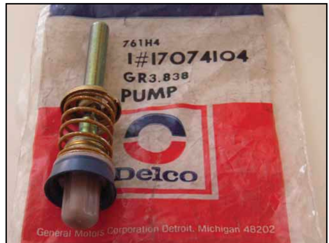
This accelerator pump from AC Delco has updated materials that will withstand today's reformulated gasoline.
