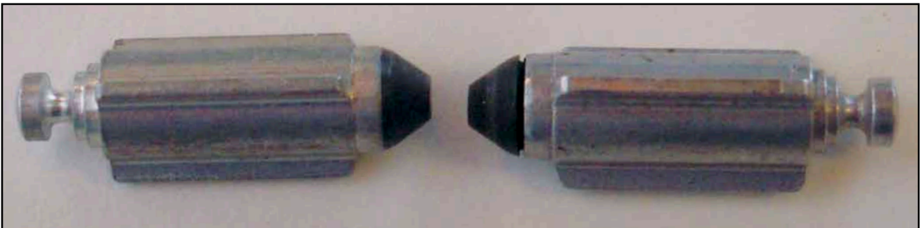
The swelling that can occur when a vintage carburetor is exposed to today's reformulated gasoline can be seen by looking at the rubber tip of the needle on the right. Compare it to the new one on the left.
