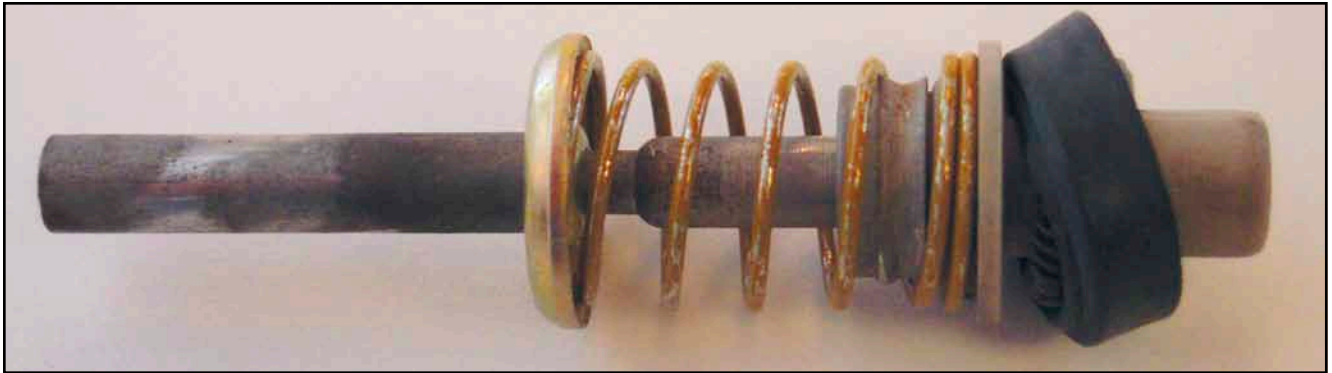
This accelerator pump failed when it was exposed to gasoline with a high level of ethanol.
