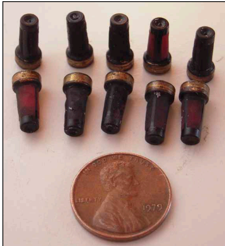
These very dirty fuel injector filters are from an engine that ran on compressed natural gas.
