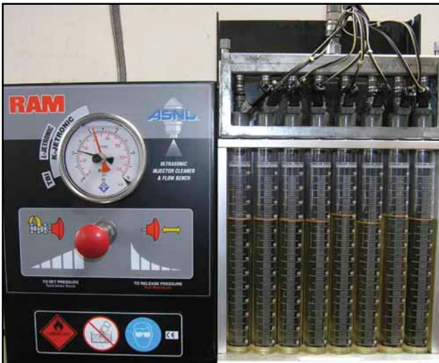
The flow from the injectors should be within 3% of each other.
