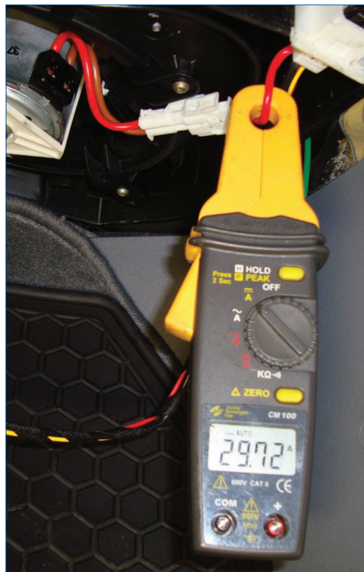
You should always check the amperage draw of the blower motor when replacing the blower module. Excessive amp draw can damage the new unit. Blower motors typically draw about 30 amps during high-speed operation.
