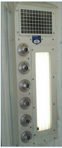
Air movement is the most important factor in drying water-borne paints. Temperature has less effect. Paint manufacturers have developed paint with improved drying times comparable to solvent-based finishes.
