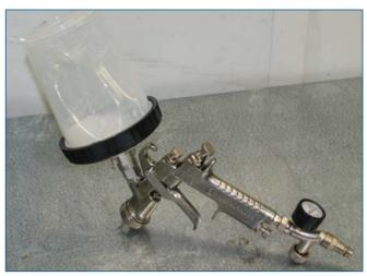
Your HVLP gun should be set to between 25 and 35 psi while applying the color coat. The regulator on the gun will allow you to precisely control this pressure. Try to stay away from metal reservoirs as they will corrode over time.
