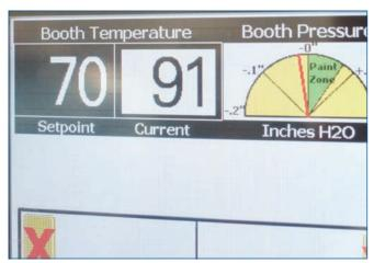
You may have to vary the settings of your paint booth to account for ambient temperature. As you can see here the temperature is set for 70 deg. F., but the actual reading is 90. Use lower temperatures for longer drying times.
